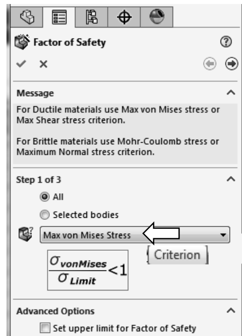
Figure 28 – The failure criterion is selected in Step 1 of 3 of the Factor of Safety dialogue box.
