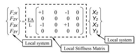
Using the equations we derived in the previous sections, the GLOBAL system equation for *Element B* is:
