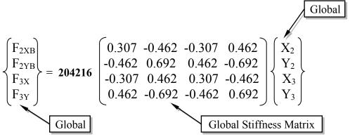
Now we are ready to assemble the overall global stiffness matrix of the structure.
