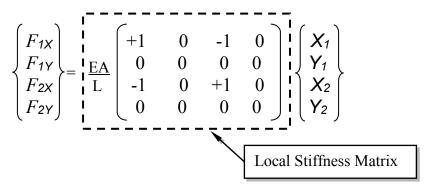
The force-displacement equations (in the local coordinate system) can be expressed as:
