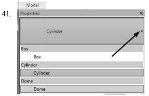
Select the **Dome** component using the Type Selector.
