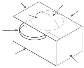
Select the four sides of the box, the outside arc of the cylinder and the two sides of the dome to place walls.
