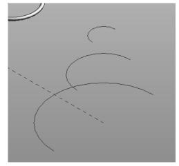
Our final shape will be a BLEND or LOFT. A blend is created using two or more open or closed sketches. Each sketch must be placed on a different reference plane or level.
