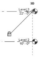
Pick to place the end point to position the level indicator above the other indicators.
