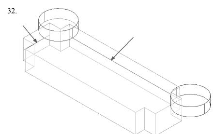
Select the two lines used to locate the circle sketch.
