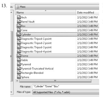
Hold down the CTRL Key and select the *Dome*, *Box*, and *Cylinder* files.
