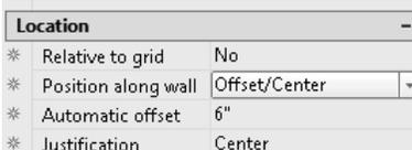
Expand the Location section in the Properties palette. Set the Position along wall to **Offset/Center**. Set the Automatic offset to **6" [300.00]**.
