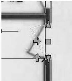
The horizontal arrow flips the orientation of the door to the other side of the wall.
