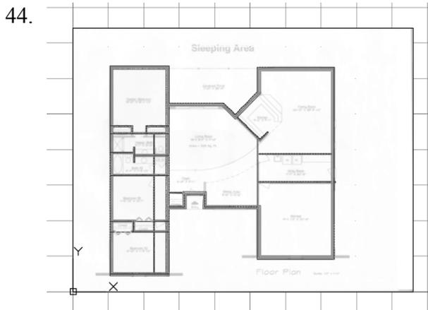
Image layer is adjusted to be faded. Dimensions were moved to a layer named A-Anno-Dim and then frozen.
