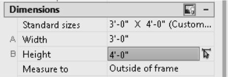
On the Properties palette, expand the Dimensions section.
