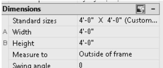
On the Properties palette, expand the Dimensions section.
