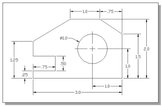
2. Spacer Plate (Thickness: .125)
