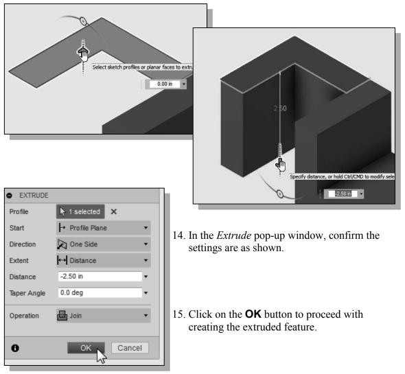
13. Drag the arrow **downward**, with the left mouse button, and set the extrusion distance to **-2.5** as shown.
