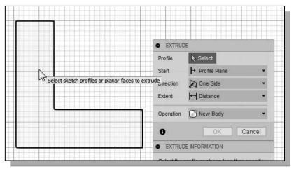
3. In the *Extrude* edit box, enter **2.5** as the extrusion distance.
