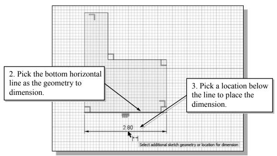
3. Move the graphics cursor below the selected line and left-click to place the dimension. (Note that the value displayed on your screen might be different than what is shown in the figure above.)
