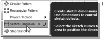
In the sketch toolbar, select the Sketch Dimension command as shown. The Sketch Dimension command is generally known as Smart Dimensioning in parametric modeling. 2. The message "Select Geometry to Dimension" is displayed in the Status Bar area at the bottom of the Fusion 360 window. Select the bottom horizontal line by left-clicking once on the line.
