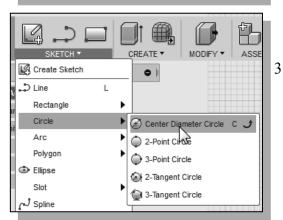
4. Create a circle of arbitrary size on the top face of the solid model as shown.
