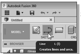
3. Select the **Line** command by clicking once with the **left-mouse-button** on the icon in the *Sketch* tab on the Ribbon.
