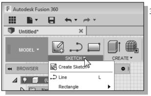
3. Click and press on the **Sketch** tab in the main *Ribbon* area to display the available sketching tools as shown. Also note the Sketch Palette panel is also activated with additional sketching options.
