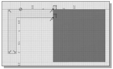
4. Create a sketch, starting at the top left corner of the solid model, with five line segments perpendicular/parallel to the solid model as shown below.
