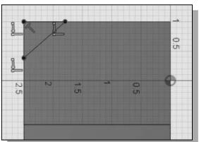
5. On your own, create and modify the two dimensions of the sketch as shown in the figure. (Hint: create the angle dimension by selecting the two adjacent lines and place the angular dimension inside the desired quadrant.)
