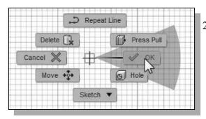
Inside the graphics window, click once with the right-mouse-button to display the option menu. Select [OK] in the pop-up menu, or hit the [Esc] key once to end the Sketch Line command.
