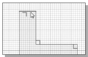
6. Select the bottom-horizontal line as the second entity to dimension as shown.
