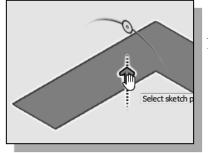
12. Move the cursor on top of the arrow; notice the dashed line appears as shown. We can drag the arrow, with the left mouse button, to set the extrusion distance and direction.
