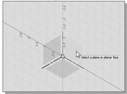
• The *sketching plane* is a reference location where two-dimensional sketches are created. Note that the *sketching plane* can be any planar part surface or datum plane.
