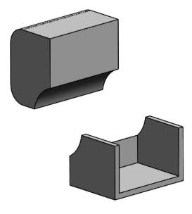
**1.10.** - Edit the "Cut-Extrude1" feature, turn the "Auto-select" option OFF in the "Feature Scope," and select the top body only. Click **OK** to finish. Now we are only cutting into the top solid, even when the cut overlaps the lower body.
