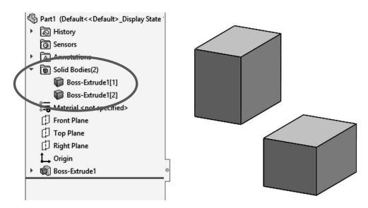
**1.3.** - The next step is to add a new feature. When working in a multi body part we can make 'local' operations to each body, in other words, a feature affecting only one solid body. Local operations are applied features like fillets, shells, chamfers, etc., which can only be applied to a single body at a time. Select the "Shell" command from the Features toolbar, and shell the bottom body removing the indicated faces.
