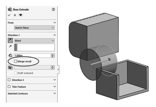
**1.7.** - After adding this extrusion we have three different bodies in our part. See how the different bodies' edges intersect each other. If the "Merge result" option had been checked, we would not see the overlapping edges as they would have merged into a single body.
