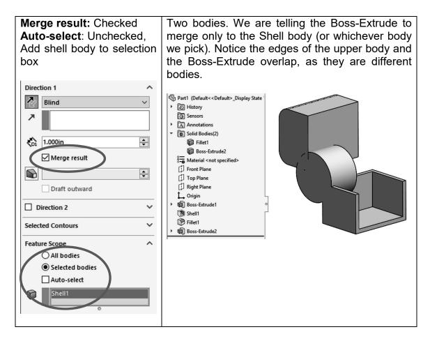
**1.8.** - The "Merge result" option works the same way with any feature that adds material to the part, including revolved boss, sweep, loft, etc. Now we'll see how it works when material is removed. Delete the last Boss-Extrude feature and keep the sketch. When deleting the "Boss-Extrude," make sure the option "Delete absorbed features" is unchecked; this way the boss will be deleted, but the sketch will be left behind.
