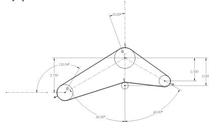
Depending on the location of the pulleys, SOLIDWORKS calculates the length for the belt automatically. Once the belt is created, the belt length can be altered and the pulleys are adjusted accordingly.
