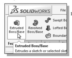
1. In the *Features* toolbar select the **Extruded Boss/ Base** command by clicking once with the left-mouse-button on the icon.
