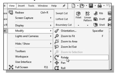
2. Move the cursor inside the graphics area. Press down the left-mouse-button and drag in an arbitrary direction; the Rotate View command allows us to freely rotate the solid model.
