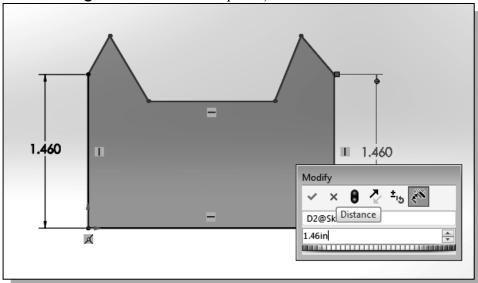
❖ The Smart Dimension command will create a length dimension if a single line is selected.
