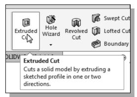
1. In the *Features* toolbar select the **Extruded Cut** command by clicking once with the left-mouse-button on the icon.
