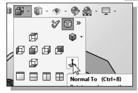
3. Adjust the display by using the **Normal To** option in the view orientation panel as shown.
