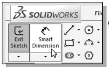
6. Select the **Smart Dimension** command in the *Sketch* toolbar. The **Smart Dimension** command allows us to quickly create and modify dimensions.
