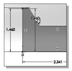
19. Select the longer inclined line on the left as the 2<sup>nd</sup> geometry to dimension.
