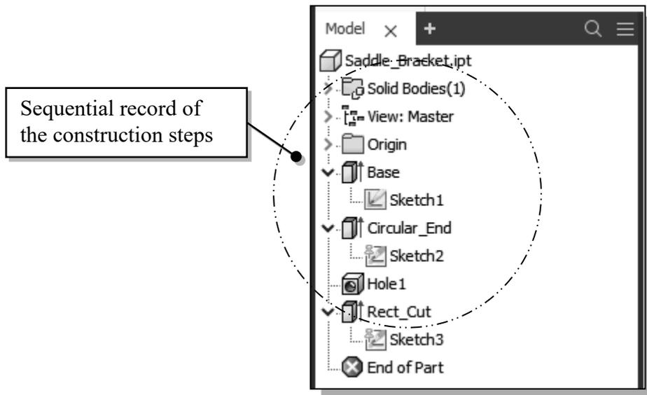
Feature-based parametric modeling is a cumulative process. Every time a new feature is added, a new result is created and the feature is also added to the history tree. The database also includes parameters of features that were used to define them. All of this happens automatically as features are created and manipulated. At this point, it is important to understand that all of this information is retained, and modifications are done based on the same input information.
