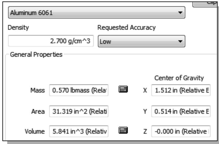
❖ Note the *General Properties* area now has the *Mass, Area, Volume* and the *Center of Gravity* information of the model based on the density of the selected material.
