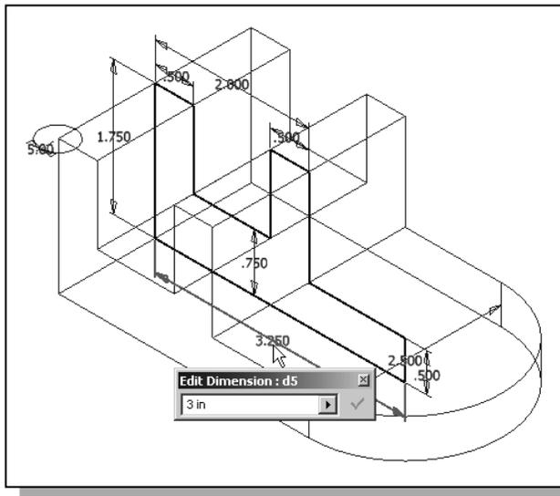
3. All dimensions used to create the **Base** feature are displayed on the screen. Select the overall width of the **Base** feature, the **3.25** dimension value, by double-clicking on the dimension text as shown.
