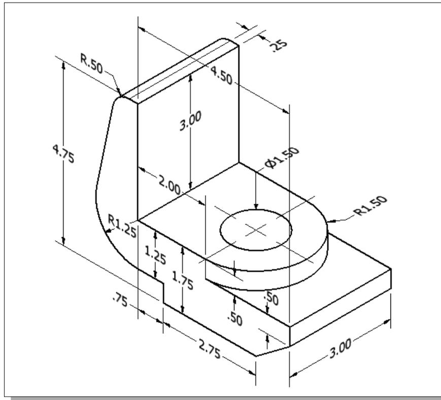
4. **Transfer Fork** (Dimensions are in inches. Material: **Cast Iron**. Volume =?)
