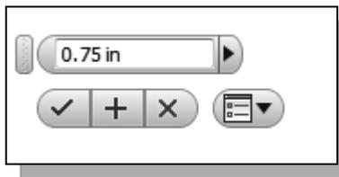
5. Set the hole diameter to **0.75 in** as shown.
