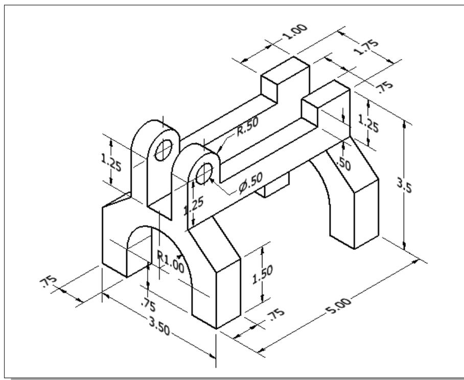
5. **Guide Slider** (Material: **Cast Iron**. Weight and Volume =?)
