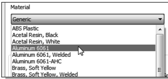
4. Click the down-arrow in the *Material* option to display the material list, and select **Aluminum-6061** as shown.
