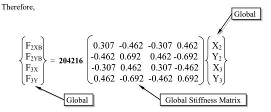
Now we are ready to assemble the overall global stiffness matrix of the structure.
