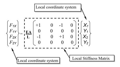
Using the equations we have derived, the GLOBAL system equations for *element* A can be expressed as:
