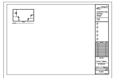
66. Highlight the Level 1 - 2000 Remodel Demo Floor plan.Hold down the left mouse button and drag the view onto the sheet. Release the left mouse button to click to place.
