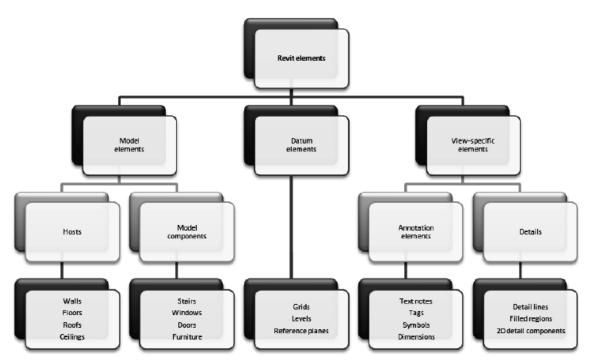
Revit elements are separated into three different types of elements: Model, Datum and View-specific. Users are expected to know if an element is model, datum or view-specific.
