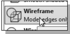
The *Wireframe Image* display option allows the display of the 3D objects using the basic wireframe representation scheme.
