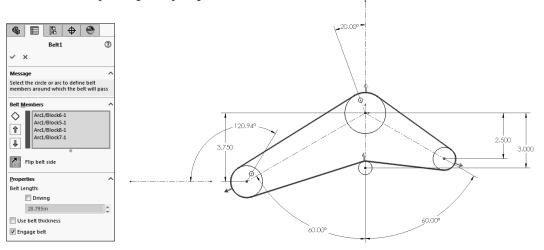
Depending on the location of the pulleys, SOLIDWORKS calculates the length for the belt automatically. Once the belt is created, the belt length can be altered and the pulleys are adjusted accordingly.
