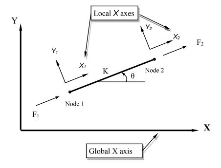
The force-displacement equations expressed in terms of components in the local XY coordinate system:
