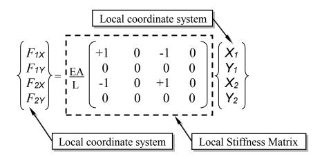
Using the equations we have derived, the GLOBAL system equations for *Element A* can be expressed as:
