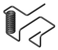
A 3D sketch normally consists of lines and arcs in series and Splines. You can use a 3D sketch as a sweep path, as a guide curve for a loft or sweep, a centerline for a loft, or as one of the key entities in a routing system.
