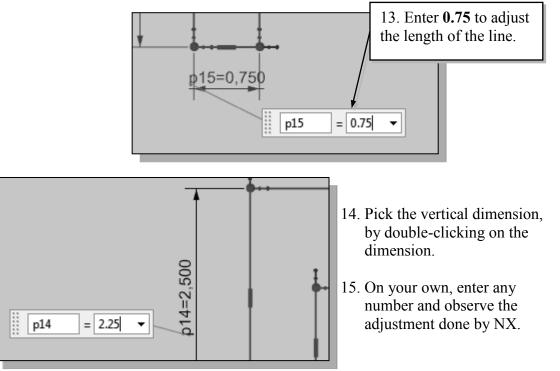
16. Inside the graphics window, hit the [**Esc**] key once to end the Rapid Dimension command.
