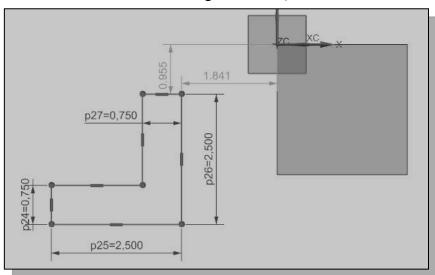
6. Modify the two unmodified location dimensions to **0.0**; this will align the position of the sketch relative to the top corner of the solid model as shown.
