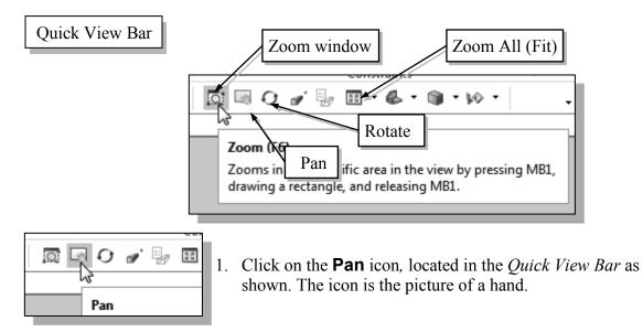
> The Pan command enables us to move the view to a different position. This function acts as if you are using a video camera.
