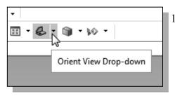
1. In *Quick View Bar*, click on the triangle icon to expand the *Orient View Drop-Down menu*.
