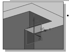
Note that the sketch plane is aligned to one of the corners of the selected face. *NX* automatically establishes a *Work-Coordinate-System* (WCS) and records its location with respect to the part on which it was created.
