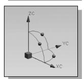
The work coordinate system (WCS) is a mobile system to assist geometric constructions in different orientations. The WCS can be located and oriented anywhere in model space.
