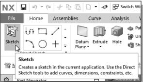
This toolbar contains tools that allow us to quickly access 2D curve options.
