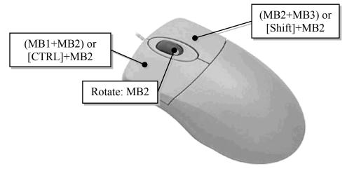
1. On your own, use the dynamic Zoom and Pan options by the mouse buttons to reposition the sketch near the center of the screen.
