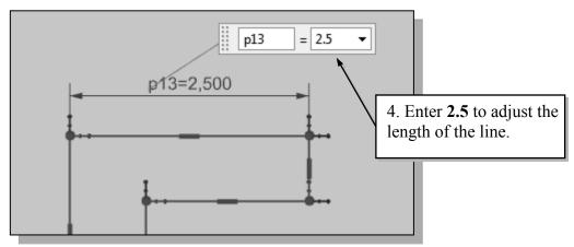
> *NX* will now update the profile with the new dimension value. Note that in parametric modeling, dimensions are used as **control variables**.
