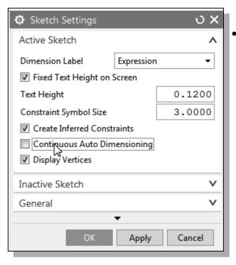
Note the different options under the *Sketch Settings* command are used during the creation of 2D sketches.
