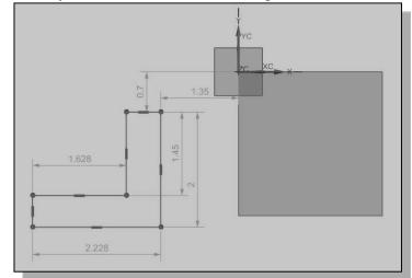
• Note that since we did not modify the **Sketch Settings**, both the *Constraints* and *dimensions* are automatically applied to the sketch.
