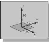
Note the default sketch plane is aligned to the XC-YC plane of the displayed *Work Coordinate System*.
