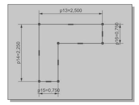
The Rapid Dimension command is also known as the Smart Dimension command; dimensions are created based on the selection of the types and orientations of objects. You might want to read through this section again and consider the powerful implication of this command. Also consider this question: How would you create an *Angle dimension* using the *Rapid Dimension* command?
