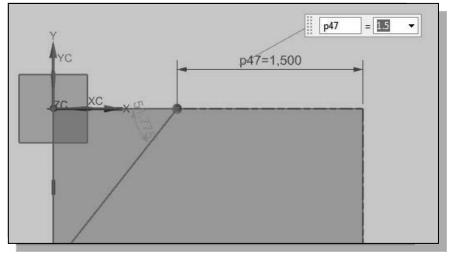
9. Select the two line segments and place the angular dimension inside the triangle to create the associated angle dimension.
