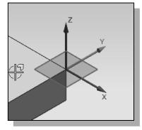
Note that the sketch plane is aligned to the selected face. *NX* automatically establishes a *Work-Coordinate-System* (WCS) and records its location with respect to the part on which it was created.
