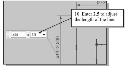
When two parallel lines are selected, the Rapid Dimension command will create a dimension measuring the distance between them.
