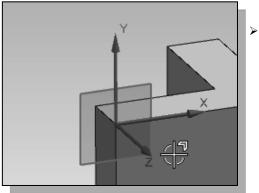
Note that the sketch plane is aligned to the selected face. *NX* automatically establishes a Work-Coordinate-System (WCS) and records its location with respect to the part on which it was created.
