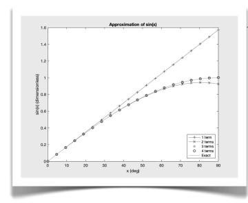
[2] Example02\_12e.m plots four approximated curves and an exact curve of sin(*x*), for comparison.  $\downarrow$
