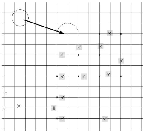
*Let's move the small circle so it is concentric to the arc using a geometric constraint.*
