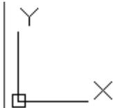
The graphics window uses a Cartesian coordinate system. The lower left corner of the screen shows a UCS (user coordinate system) icon. The icon shows x for horizontal and y for vertical. The z-axis is pointed toward the user. The UCS is located at the 0,0 or origin point.
