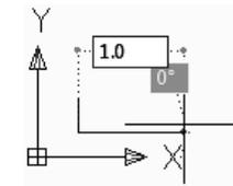
You should see another geometric constraint. This symbol indicates that the two lines are perpendicular to each other. Perpendicular means two lines form a 90° angle.
