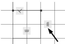
*You can only apply a vertical constraint if the perpendicular constraint has been removed. Too many geometric constraints on the same element is not allowed.*
