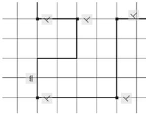
The perpendicular constraints on the selected line are deleted.
