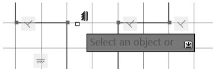
*You will see the Vertical constraint icon and a prompt to select the element where the constraint is to be applied.*
