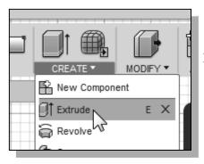
1. In the *Create toolbar*, select the **Extrude** command by clicking the left-mouse-button on the icon as shown.
