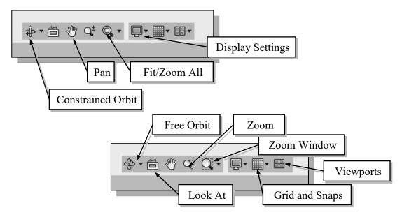
**Orbit** – In a part or assembly, adds an orbit symbol and cursor to the view. You can orbit the view planar to the screen around the center mark, around a horizontal or vertical axis, or around the X and Y axes.
