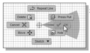
2. Inside the graphics window, click once with the **right-mouse-button** to display the option menu. Select [**OK**] in the pop-up menu, or hit the [**Esc**] key once to end the **Sketch Line** command.
