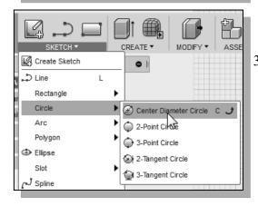
4. Create a circle of arbitrary size on the top face of the solid model as shown.
