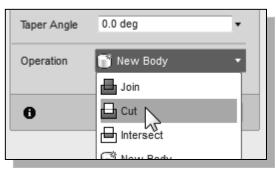
11. Select the **CUT** option in the *feature option* list to set the extrusion operation to *Cut*.
