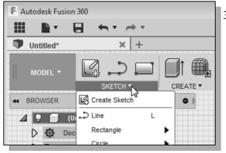
3. Click and press on the **Sketch** tab in the main *Ribbon* area to display the available sketching tools as shown. Also note the **Sketch Palette** panel is also activated with additional sketching options.
