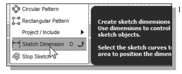
1. In the sketch toolbar, select the Sketch Dimension command as shown. The Sketch Dimension command is generally known as **Smart Dimensioning** in parametric modeling.
