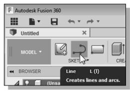
3. Select the **Line** command by clicking once with the **left-mouse-button** on the icon in the *Sketch* tab on the Ribbon.
