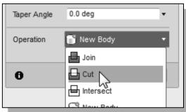
10. Select the **CUT** option in the *feature option* list to set the extrusion operation to *Cut*.
