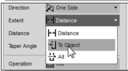
11. Set the *Extents* option to **To Object** as shown. The *To Object* option instructs the software to calculate the extrusion distance and assures the created feature will always cut through the proper length of the model.
