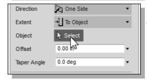
Note the Select icon is activated and Fusion 360 expects us to select an object to set the termination of the extrude feature.
