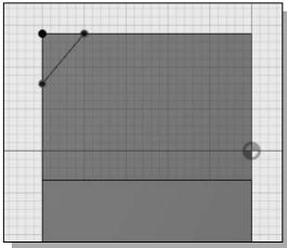
4. Start at the upper left corner and create **three line segments** to form a small triangle as shown.
