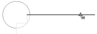
Locate the midpoint of the small horizontal line and pick.
