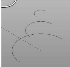
Our final shape will be a BLEND or LOFT. A blend is created using two or more open or closed sketches. Each sketch must be placed on a different reference plane or
