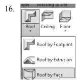
Select the **Roof by Face** tool on the Build panel on the Architecture ribbon.
