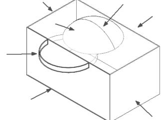
Select the four sides of the box, the outside arc of the cylinder and the two sides of the dome to place walls.
