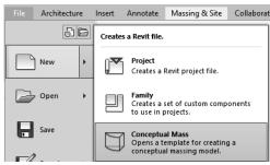
Create an extrude, revolve, sweep and blend using New→Conceptual Mass from the Applications menu.
