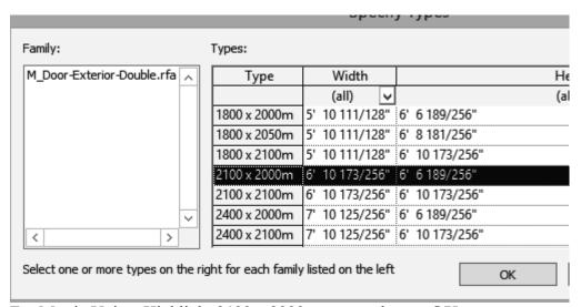
For Metric Units: Highlight 2100 x 2000m type and press OK.
