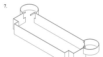
Select each wall and cylinder. The cylinder will be halved by the walls, so you will have to select each half.
