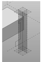
Hold down the CONTROL key and select the Axis Line (this is a reference line) and the sketch.
