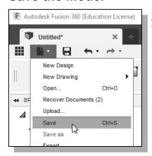
1. Select **Save** in the *Quick Access* toolbar, or you can also use the "**Ctrl-S**" combination (hold down the "Ctrl" key and hit the "S" key once) to save the part.
