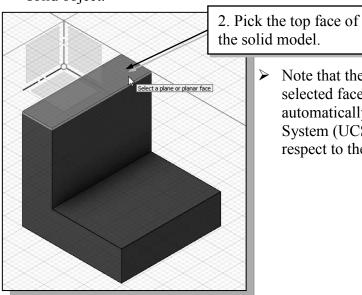
Note that the sketch plane is aligned to the selected face. Autodesk Fusion 360 automatically establishes a User-Coordinate-System (UCS) and records its location with respect to the part on which it was created.
