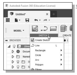
3. Click and press on the **Sketch** tab in the main *Ribbon* area to display the available sketching tools as shown. Also note the **Sketch Palette** panel is also activated with additional sketching options.
