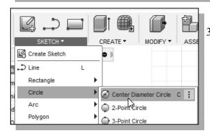
3. Select the **Center Diameter circle** command by clicking once with the **left-mouse-button** on the icon in the *Sketch* toolbar as shown.
