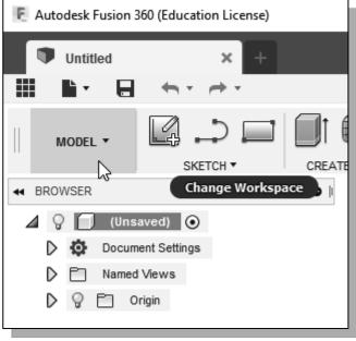
Autodesk Fusion 360 is an integrated system that can be used to create parts, assembly, animation, simulation, CAM and 2D drawings. By default, the **Model WorkSpace** is activated as shown.
