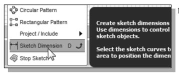
In the sketch toolbar, select the Sketch Dimension command as shown. The Sketch Dimension command is generally known as Smart Dimensioning in parametric modeling. 2. The message "Select Geometry to Dimension" is displayed in the Status Bar area at the bottom of the Fusion 360 window. Select the bottom horizontal line by left-clicking once on the line.
