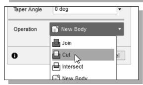
11. Select the **CUT** option in the *feature option* list to set the extrusion operation to *Cut*.
