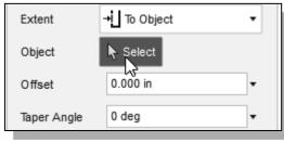
Note the Select icon is activated and Fusion 360 expects us to select an object to set the termination of the extrude feature.
