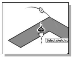
12. Move the cursor on top of the arrow; notice the dashed line appears as shown. We can drag the arrow, with the left mouse button, to set the extrusion distance and direction.
