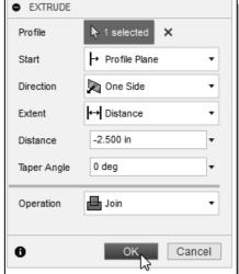
14. In the *Extrude* pop-up window, confirm the settings are set to **Join** and **-2.50** in as shown.
