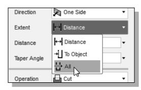
14. Set the *Extent* option to **Through All** as shown. The *All* option instructs the software to calculate the extrusion distance and assures the created feature will always cut through the full length of the model.
