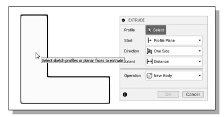
3. In the *Extrude* edit box, enter **2.5** as the extrusion distance.
