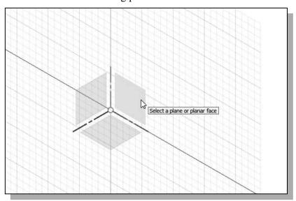
• The *sketching plane* is a reference location where two-dimensional sketches are created. Note that the *sketching plane* can be any planar part surface or datum plane.
