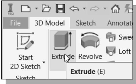
11. In the *3D Model* tab, select the **Extrude** command by clicking the left-mouse-button on the icon.
