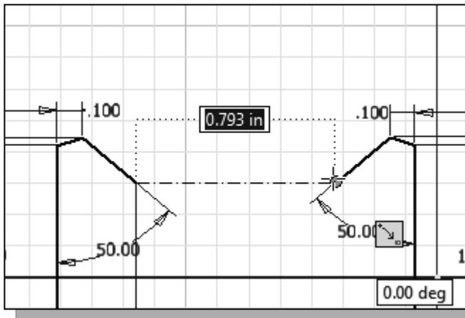
4. Move the cursor above the two selected points to set the curvature of the arc, **left-clicking** once when the radius is curved upward as shown.
