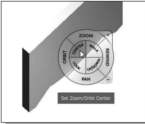
6. Move the cursor to the left side of the model and click the **Center** option as shown. The display is adjusted so the selected point is the new **Zoom/Orbit** center.
