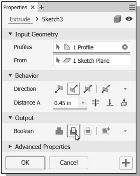
9. Click on the **CUT** icon, as shown, to set the extrusion operation to **Cut**.
