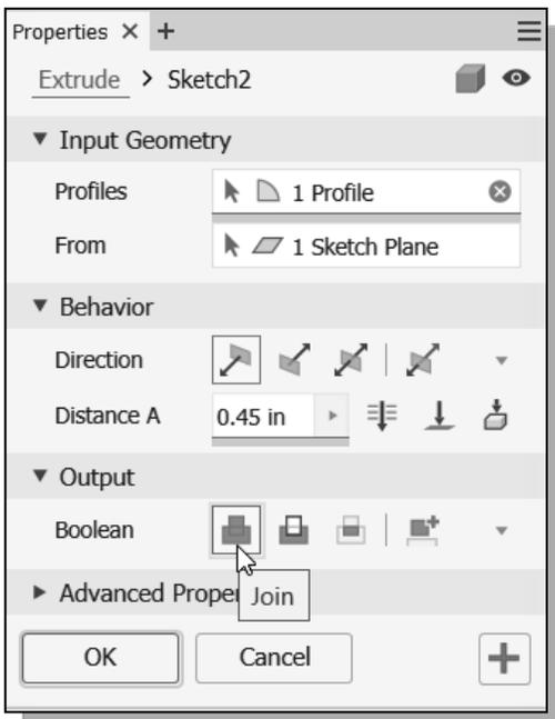
13. In the *Extrude* control panel enter **0.45** as the extrude distance as shown.
