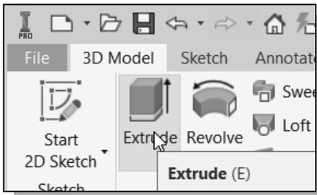
8. In the *3D Model tab* select the **Extrude** command by left-clicking on the icon.
