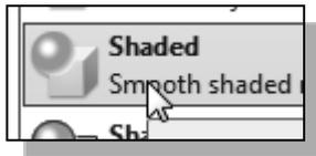
The *Standard Shaded Solid* display option generates a shaded image of the 3D object that requires fewer computer resources compared to the realistic rendering.
