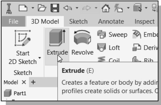
1. In the 3D Model tab (the tab is located in the **Ribbon**) select the **Extrude** command by clicking the left-mouse-button on the icon.
