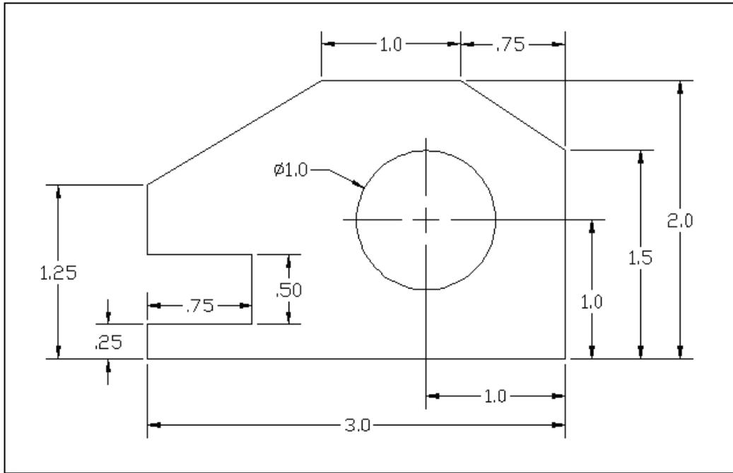
2. **Spacer Plate** (Thickness: .125)
