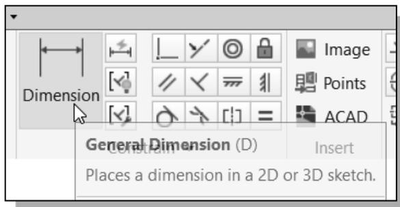
1. Move the cursor to the *Constrain* toolbar area; it is the toolbar next to the 2D *Draw* toolbar. Note the first icon in this toolbar is the **General Dimension** icon. Left-click once on the icon to activate the **Dimension** command.
