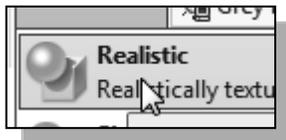
The *Realistic Shaded Solid* display mode generates a high quality shaded image of the 3D object.
