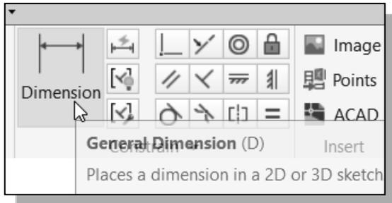
5. Left-click once on the icon to activate the **General Dimension** command. The *General Dimension* command allows us to quickly create and modify dimensions.
