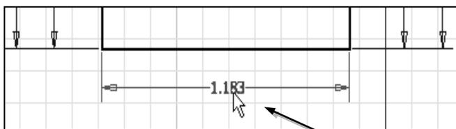
1. Select the dimension that is at the bottom of the sketch by **double-clicking** on the dimension text.
