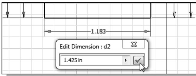
2. In the *Edit Dimension* window, the current length of the line is displayed. Enter **1.425** to set the length of the line.
