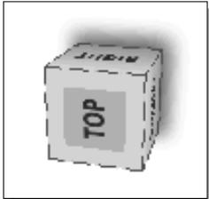
9. Move the cursor over the ViewCube and drag with the left-mouse-button to activate the **Free Rotation** option.
