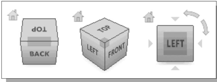
Once the ViewCube is displayed, it is shown in one of the corners of the graphics window over the model in an inactive state. The ViewCube also provides visual feedback about the current viewpoint of the model as view changes occur. When the cursor is positioned over the ViewCube, it becomes active and allows you to switch to one of the available preset views, roll the current view, or change to the Home view of the model.
