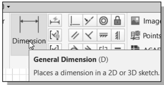
5. Select the **General Dimension** command in the *Constrain* toolbar. The **General Dimension** command allows us to quickly create and modify dimensions. Left-click once on the icon to activate the **General Dimension** command.
