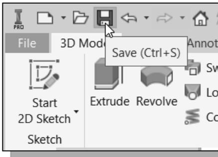
1. Select **Save** in the *Quick Access* toolbar, or you can also use the “**Ctrl-S**” combination (hold down the “**Ctrl**” key and hit the “**S**” key once) to save the part.
