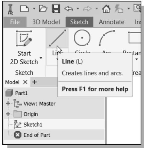
1. Move the graphics cursor to the **Line** icon in the *Draw* toolbar. A *Help tip* box appears next to the cursor and a brief description of the command is displayed at the bottom of the drawing screen: “Creates Straight line segments and tangent arcs.”
