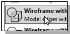
The *Wireframe with Hidden-Edge Display* option can be used to generate an image of the 3D object with all the back lines hidden.
