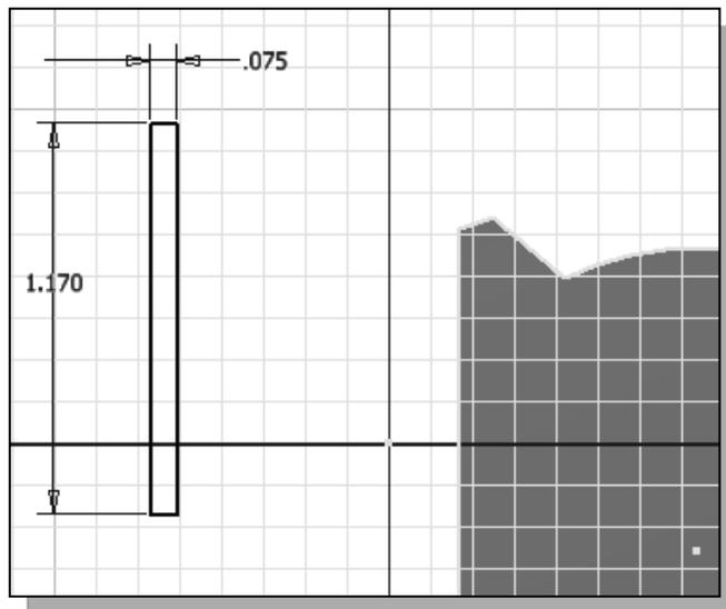
6. The message “*Select Geometry to Dimension*” is displayed in the *Status Bar* area at the bottom of the Inventor window. Create and modify the size dimensions to describe the size of the sketch as shown in the figure.
