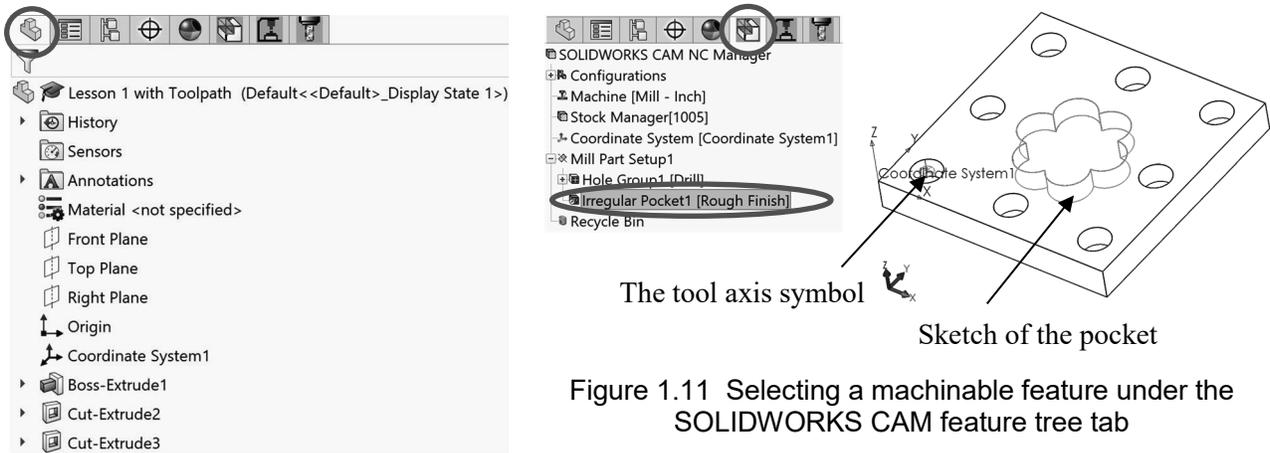
Figure 1.11 Selecting a machinable feature under the SOLIDWORKS CAM feature tree tab
