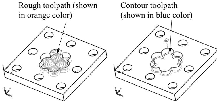
Figure 1.4 Toolpath of the pocket milling operations
