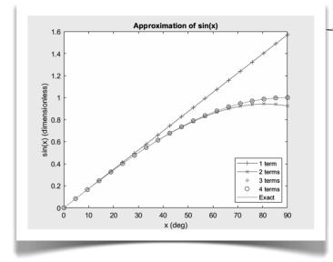
[2] Example02\_12e.m plots four approximated curves and an exact curve of sin(x), for comparison.  $\downarrow$
