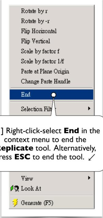
[12] We chose to manually set the paste handle at a vertex ([3-4], last page) because we want to demonstrate the use of **Set Paste Handle** [3]. In this case, select **Use Plane Origin as Handle, Rotate by r**, and then **Paste at Plane Origin** have the same result. #
