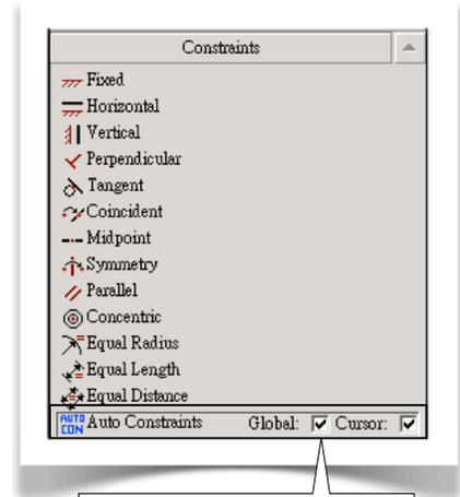
[2] By default, DesignModeler is in the **Auto Constraints** mode, both globally and locally. #
