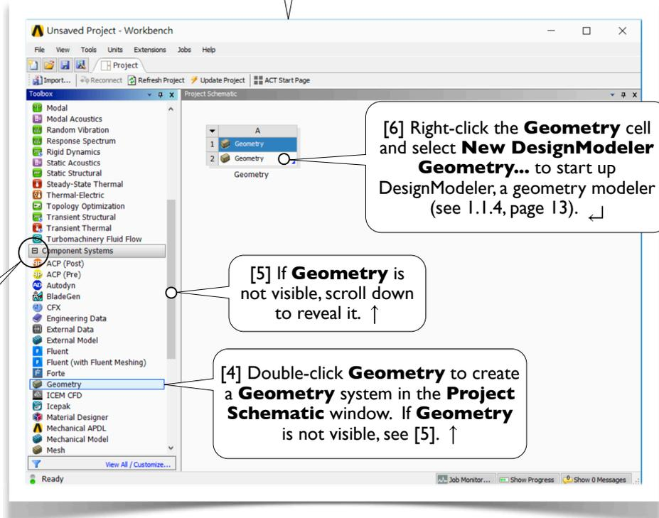
[6] Right-click the **Geometry** cell and select **New DesignModeler Geometry...** to start up DesignModeler, a geometry modeler (see 1.1.4, page 13). ✓
