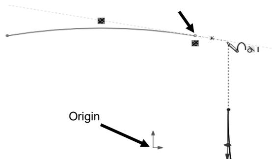
4. Drag the **pointer to the right** so it's tangent with the arc. Because the endpoint is attached to the existing arc sketch, a yellow inferencing line is displayed.
