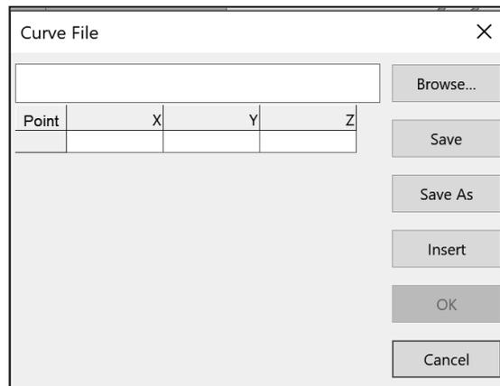
Create a curve using the Curve Through XYZ Points tool. Import the x-, y-, z- data. Verify that the first and last points in the curve file are the same for a closed profile.
