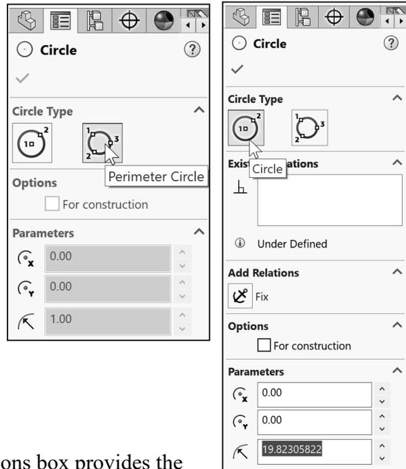
The Perimeter Circle Sketch entity provides the ability to define a circle using 3 points along its perimeter. This sketch entity is very useful when you are not concerned about the location of the center of the circle.
