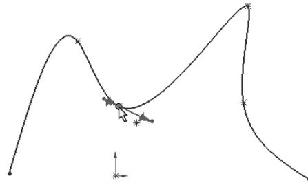
Modify the Spline shape using the click and drag method on a handle.
