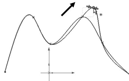
Modify the Spline shape using the x-, y- and z- coordinates method on a control point.
