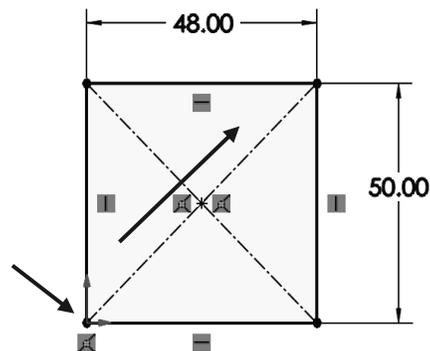
Create the first feature for the model. The Extruded Boss/Base feature adds material to a part. Extrude the sketch to create the first feature. Apply symmetry.
