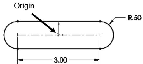
Apply the Instant3D tool. Create an Extruded Boss/Base feature. The Extruded Boss/Base feature adds material to a part. Note: Edit the feature, and view the PropertyManager to confirm that you picked the correct dimension with the on-screen ruler. The Instant3D tool does not provide various End Conditions for Design Intent.
