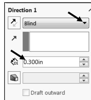
Create an Extruded Cut feature using Instant3D.
