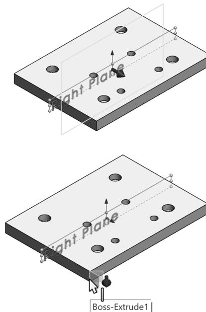
6. Click the **front vertical edge** of Extrude1 as illustrated. Do not select the midpoint. Edge<1> is displayed in the Selections box. The model is fully defined.
