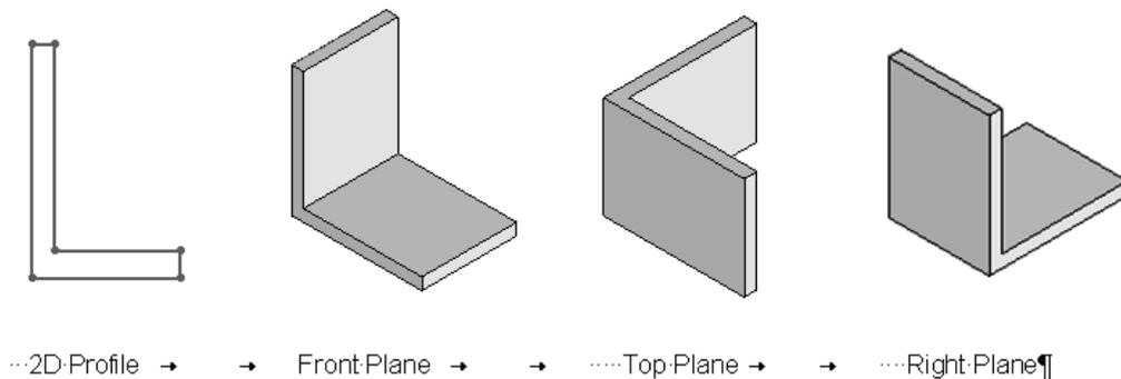
The six principle views of Orthographic projection listed in the ASME Y14.3 2009 standard are *Front, Top, Right, Bottom, Rear, and Left*. SOLIDWORKS Standard view names correspond to these Orthographic projection view names.
