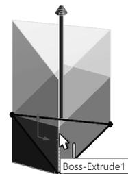
16. Click the **front right vertical edge** as illustrated to remove the material. Edge<1> is displayed in the Direction of Extrusions box.
