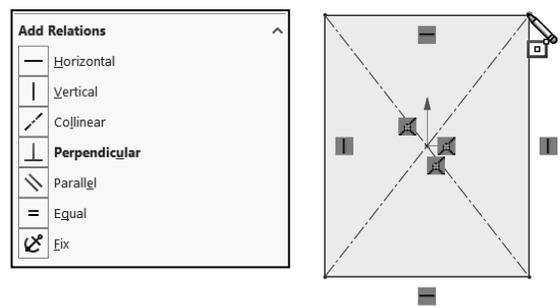
Example A: Apply design intent to create a square profile. Sketch a rectangle. Apply the Center Rectangle Sketch tool. Note: No construction reference centerline or Midpoint relation is required with the Center Rectangle tool. Insert dimensions to fully define the sketch.
