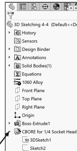
The main advantage of the 3D Sketch placement method is that it can place a set of holes on any set of solid faces, regardless of whether they are at different levels, or are non-parallel. A limitation: 3D sketches can be fairly cumbersome and difficult. See section on 3D Sketching in SOLIDWORKS Help for additional details.
