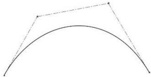
With the Style Spline tool, you can control the degree and continuity of the curves. You can inference style splines for tangency or equal curvature. You can constrain the points and dimension the curves' sides. These curves also support mirroring and self-symmetry.
