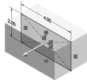
Example A: The Extruded Base feature remains symmetric about the Front Plane. Utilize the Mid Plane End Condition option in Direction 1. Modify the depth, and the feature remains symmetric about the Front Plane.
