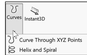
Import x-, y-, z- data. Verify that the first and last points in the curve file are the same for a closed profile.
