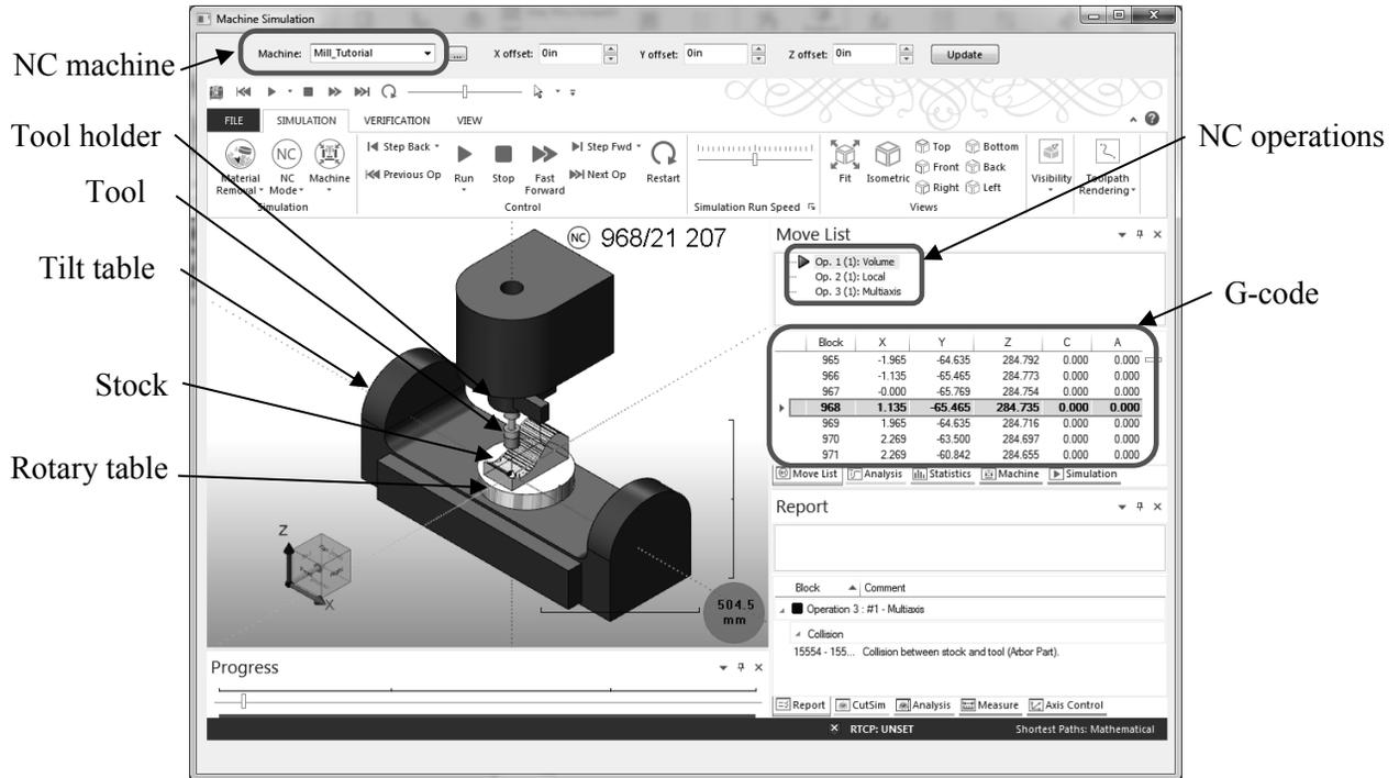
Figure 1.17 The Machine Simulation window of Mill\_Tutorial
