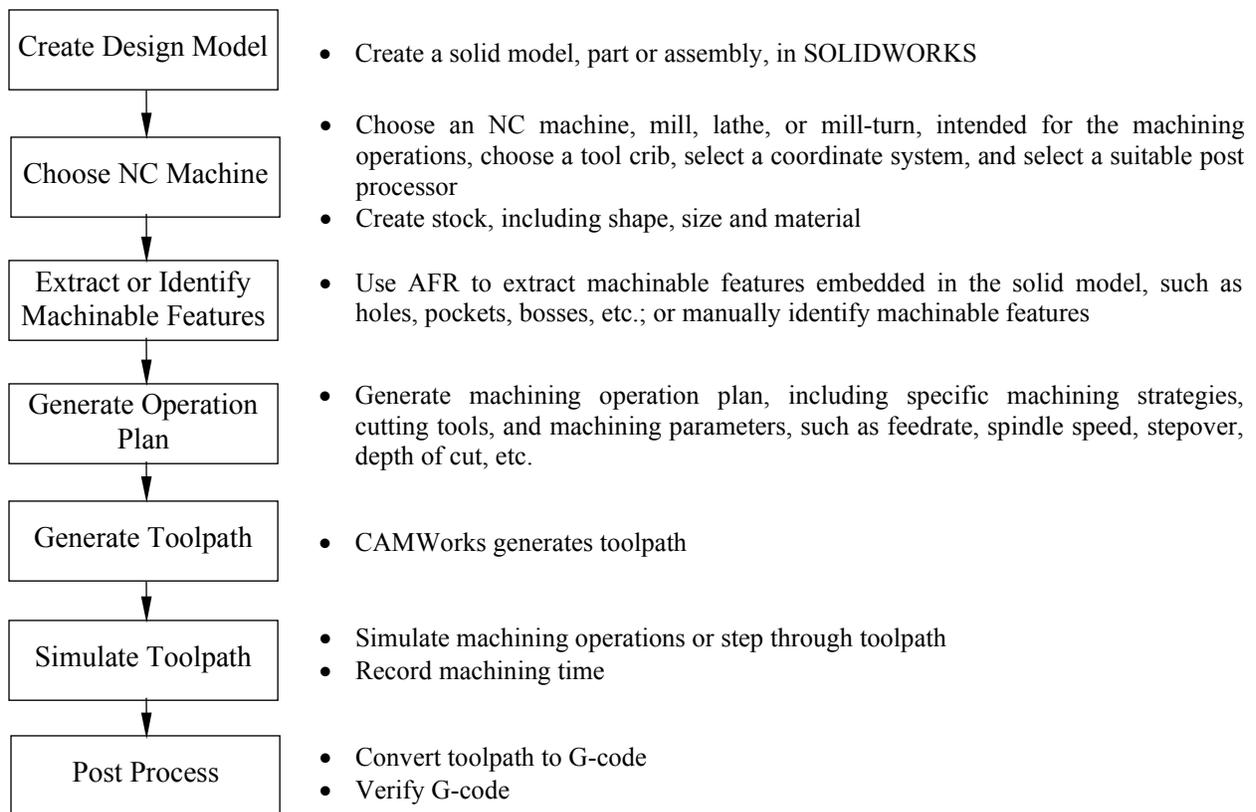
Figure 1.1 Process of conducting virtual machining using CAMWorks
