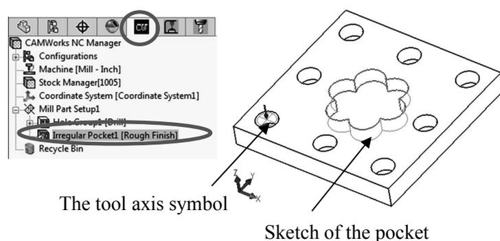
Figure 1.11 Selecting a machinable feature under the CAMWorks feature tree tab
