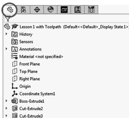
Figure 1.10 Solid features listed in the feature manager window under the FeatureManager design tree
