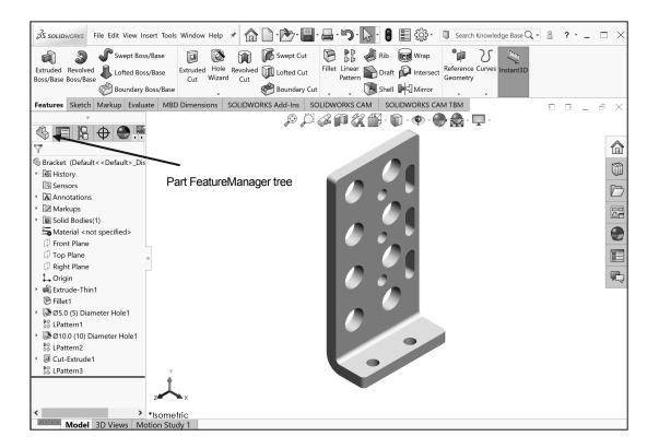
The FeatureManager design tree is located on the left side of the SOLIDWORKS Graphics window. The FeatureManager provides a summarized view of the active part, assembly, or drawing document. The tree displays the details on how the part, assembly or drawing document was created.
