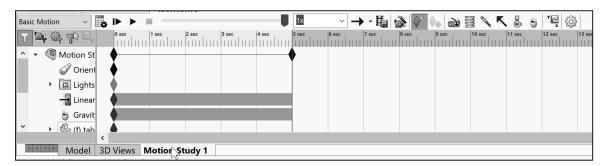
Incorporate visual properties such as lighting and camera perspective. Click the Motion Study tab to view the MotionManager. Click the Model tab to return to the FeatureManager design tree.
