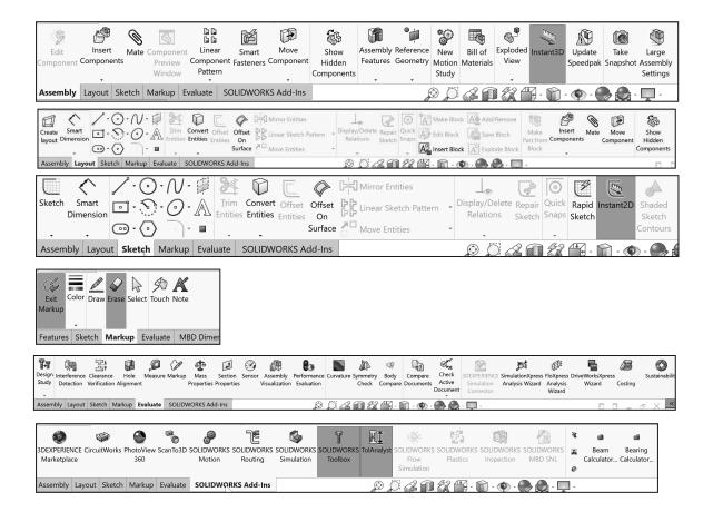
The Ink Markup toolbar is renamed to the Markup toolbar. The Markup tab is displayed by default in the CommandManager on some systems. You can draw markups with a mouse on non-touch devices, display bounding boxes for markups, create markups in drawings, and use the context toolbar to access markup options.
