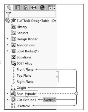
Use Dynamic reference visualization for a part, assembly and mates.
