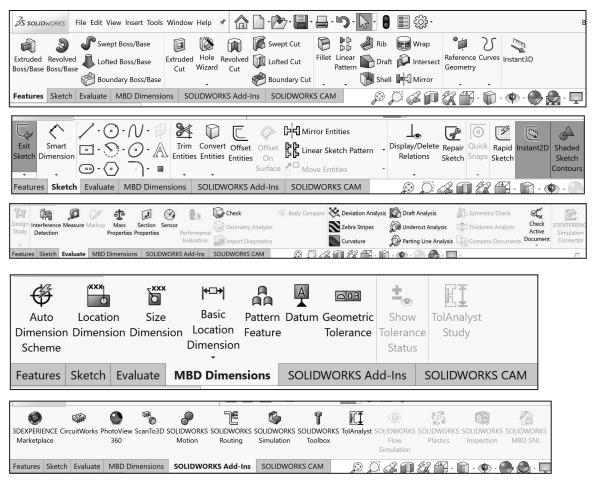
Set button size from the Toolbars tab of the Customize dialog box. To facilitate element selection on touch interfaces such as tablets, you can set up the larger Size buttons and text from the Options menu (Standard toolbar).
