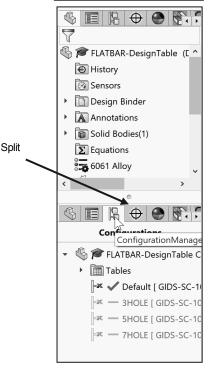
The ConfigurationManager tab is located to the right of the PropertyManager tab. Use the ConfigurationManager to create, select and view multiple configurations of parts and assemblies.
