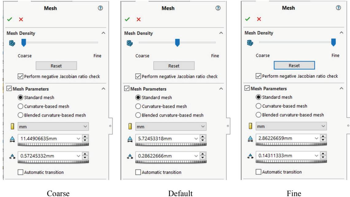
Figure 2-15: Three choices of mesh size from left to right: coarse, medium (default), and fine.
