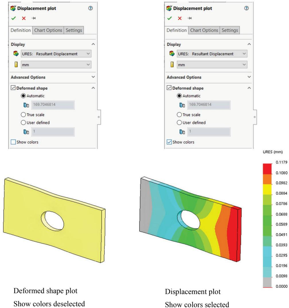
**Figure 2-26: Deformation plot (left) and Displacement plot (right).**
