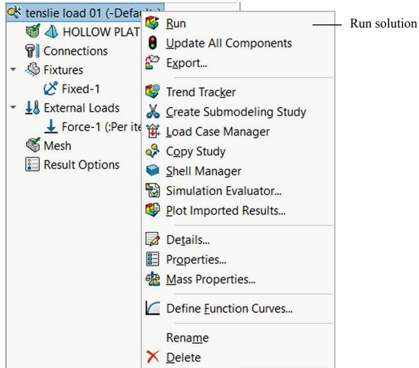
Figure 2-19: Pop-up menu for the *tensile load 01* folder.
