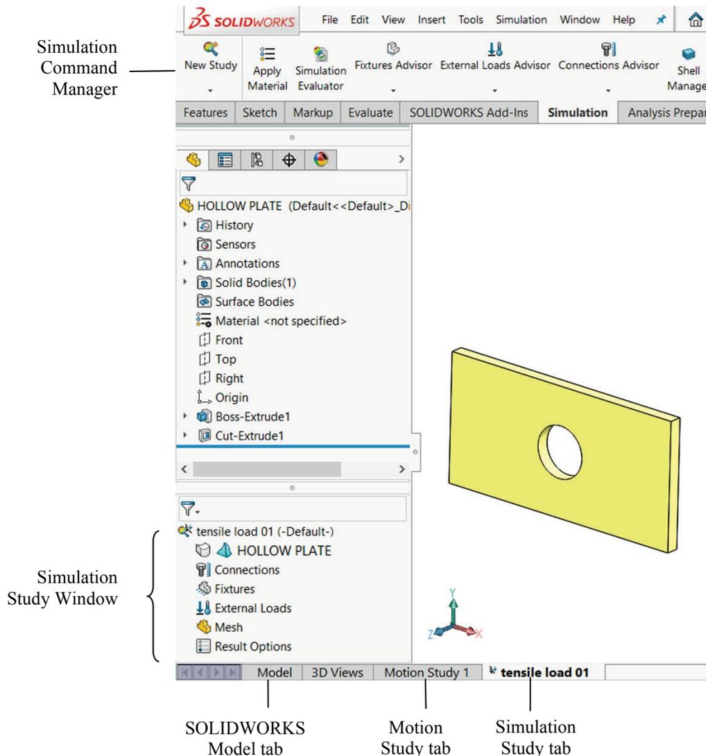
**Figure 2-7: The Simulation window and Simulation tab.**
