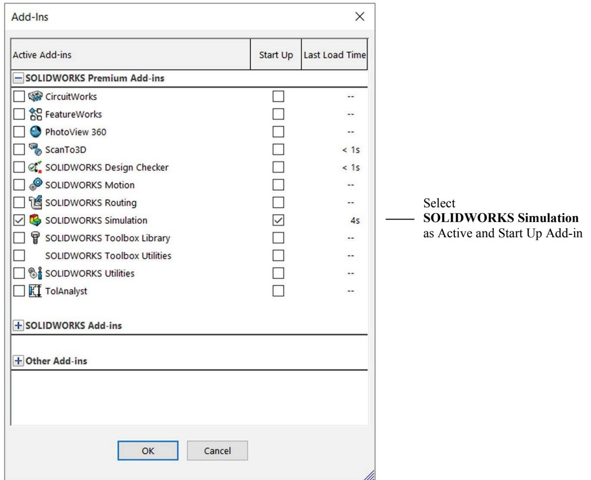
**Figure 2-2: Add-Ins list in SOLIDWORKS.**
