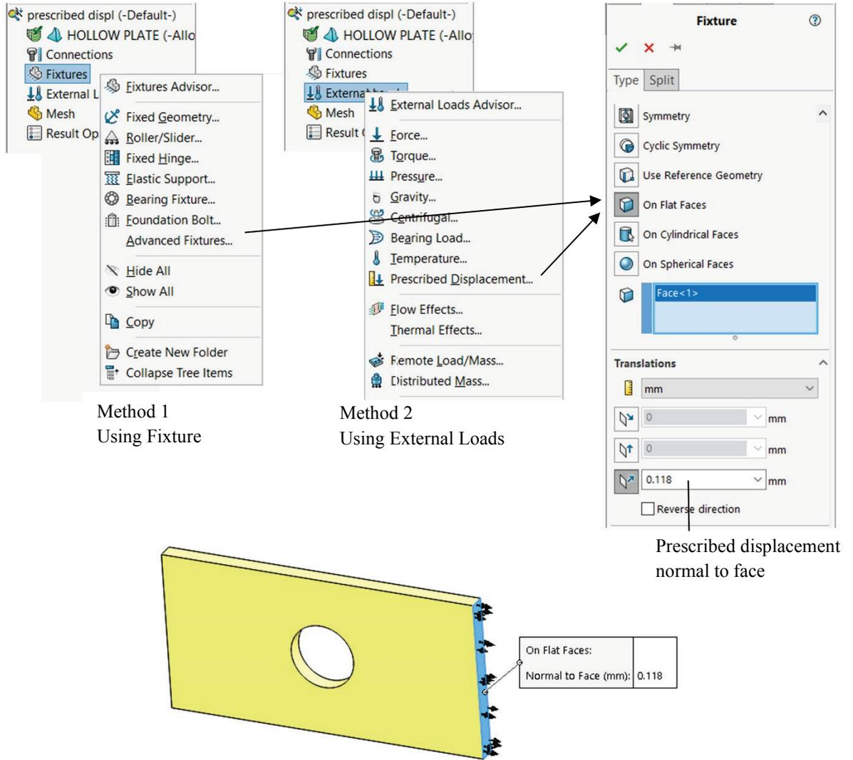
**Figure 2-37: Two methods of defining prescribed displacement.**
