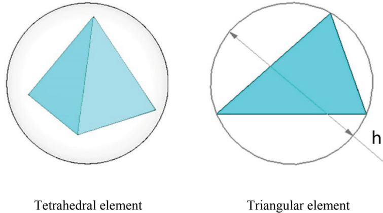
Figure 2-16: Characteristic element size of a tetrahedral element (left) and triangular element (right).
