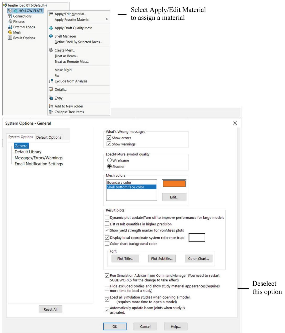
Figure 2-8: Assigning material properties.
