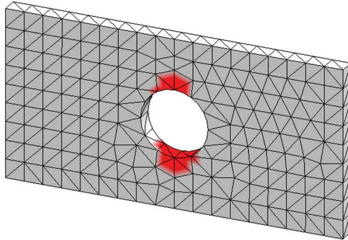
Figure 2-29: The red color displays the areas where the factor of safety falls below 3. Irregular shape of these areas is caused by the coarse mesh used in this study.
