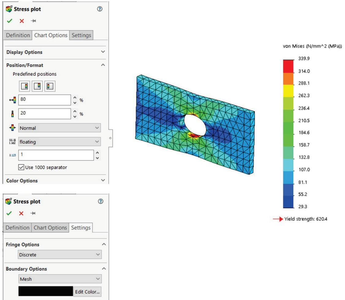
Figure 2-25: A modified stress plot is shown with floating numerical format with one decimal place as selected in Chart Options and with discrete fringes and the mesh superimposed on the stress plot as selected in Settings.
