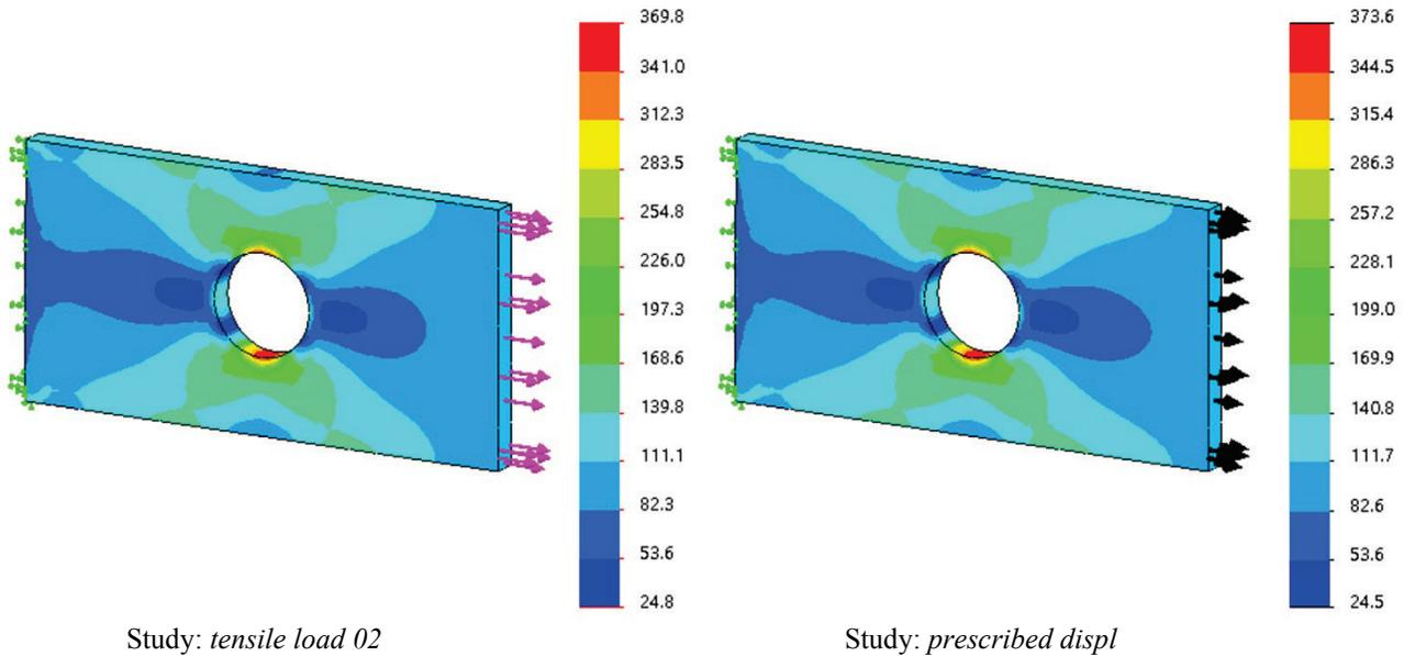
Figure 2-38: Comparison of von Mises stress results.
