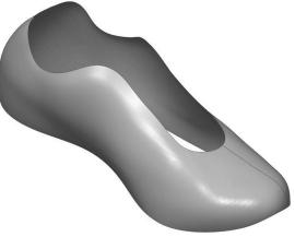
Surfaces can be used as reference geometry in order to assist with the construction of a model. The surfaces will then be moved into a Surface Bodies folder and become hidden when the model is complete.
