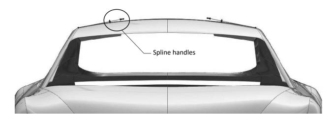
Each Spline includes a set of tools to assist with the manipulation of its curvature. These tools are: Tangent Radial **Tangent Magnitude** Handle (Translate) Handle (Rotate) Curvature Combs \* Both. Translate & \* Spline Handles **Rotate Handle** \* Inflection Points **Control Polygons** \* **Inflection Point** Curvature Combs **Spline Handles Control Polygon**
