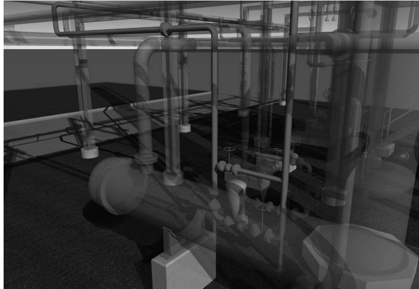
1.8 3D CAD Model of a Process Piping Design. Image Courtesy of Mustang Engineering L.P.
