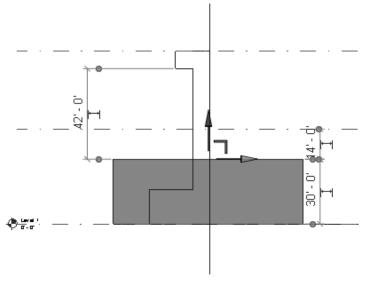
You can see how the dimensions are indicating the relative distances between the top face and the upper level, the bottom face, and another sketch.
