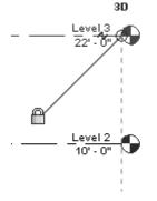
Pick to place the end point to position the level indicator above the other indicators.
