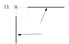
Select the two lines indicated to be used for object tracking to locate the center of the circle.
