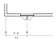
The arrows appear on the exterior side of the window. If the window is not placed correctly, left click on the arrows to flip the orientation.
