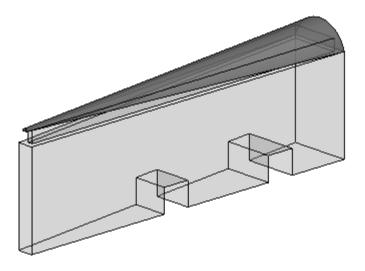
3) Make a conceptual mass family as shown. Use Solid Void to create the two openings.
