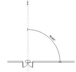
Select the center of the door as the start point of the mirror axis.
