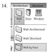
Select the **Wall by Face** tool from the Architecture tab on the ribbon.
