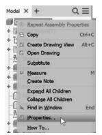
A frequent source for the answer you need is the iProperties dialog. It can be accessed by a right-click on the model in the browser. The iProperties dialog has seven tabs. The one you will need information from is the Physical tab. The physical tab offers the Mass, Volume, and Center of Gravity information on the model. When you first enter the tab that data might not be displayed. Simply click the Update button to process the
