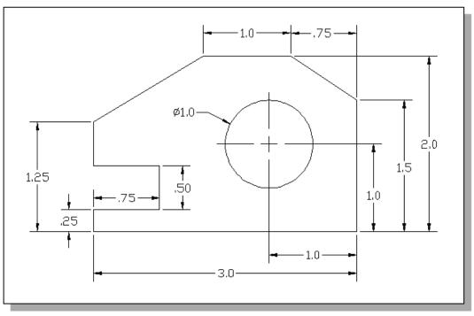
2. Spacer Plate (Thickness: .125)
