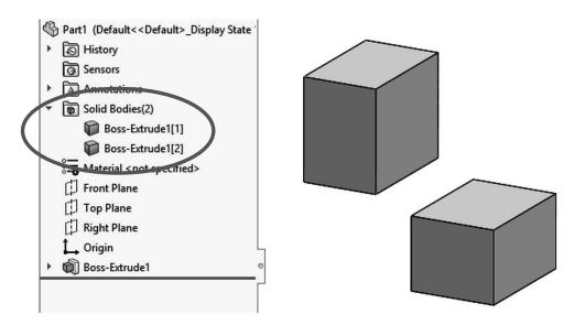
**1.3.** - The next step is to add a new feature. When working in a multi body part we can make 'local' operations to each body, in other words, a feature affecting only one solid body. Local operations are applied features like fillets, shells, chamfers, etc., which can only be applied to a single body at a time; for example, we cannot fillet or shell both bodies at the same time. Select the "**Shell**" command from the Features toolbar and shell the bottom body removing the indicated faces.
