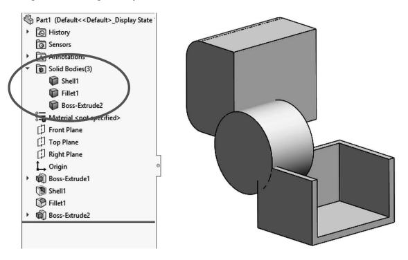
Edit the last extrusion to explore the effect of different "Merge Result" and "Feature Scope" combinations.
