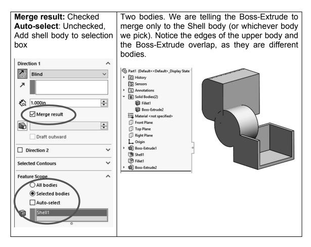
**1.8.** - The "Merge result" option works the same way with any feature that adds or removes material to the part, including revolved boss, sweep, loft, etc. Now we'll see how it works when material is removed. Delete the last Boss-Extrude feature and keep the sketch. When deleting the "Boss-Extrude," make sure the option "Delete absorbed features" is unchecked; this way the boss will be deleted, but the sketch will be left behind.
