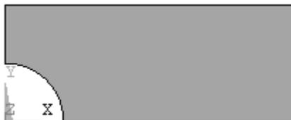
Figure 2-13 Geometry for quadrant of plate.
