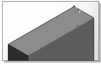
2. Move the cursor over the rear top vertex of the model. When the Coincident relation symbol appears as shown, click once with the left-mouse-button. This will start the first line, constraining its endpoint to be coincident with the vertex.
