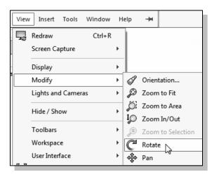
The Rotate View command allows us to rotate a part or assembly in the graphics window. Rotation can be around the center mark, free in all directions, or around a selected entity (vertex, edge, or face) on the model.
