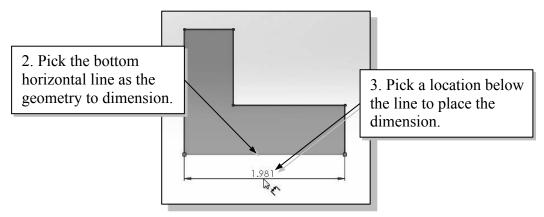
3. Move the graphics cursor below the selected line and left-click to place the dimension. (Note that the value displayed on your screen might be different than what is shown in the figure above.)
