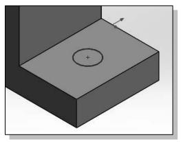
5. Create a circle of arbitrary size on the top face of the solid model as shown. Click once with the left-mouse-button to select the center of the circle, move and click again to set the radius. Press the [Esc] key once to end the Circle command.
