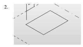
The most basic mass form is an extrude. This mass form requires a single closed polygonal sketch.
