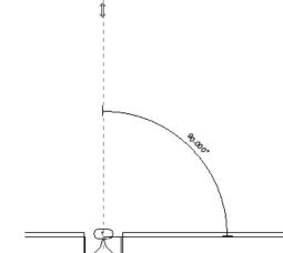
Select the center of the door as the start point of the mirror axis.
