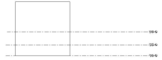
To adjust the horizontal position of the level lines, simply select the line and use the grip to extend or shorten it.
