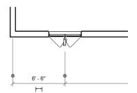
The arrows appear on the exterior side of the window. If the window is not placed correctly, left click on the arrows to flip the orientation.
