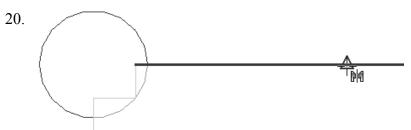
Locate the midpoint of the small horizontal line and pick.
