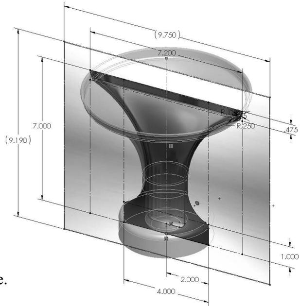
Use the Front plane and create a section view to verify the thickness of the revolved part. Exit the section view when you are done viewing.
