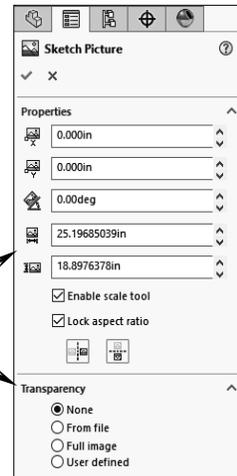
The lower left corner of the picture is placed on the origin by default, and the picture's properties appear displaying the options for moving, rotating, and scaling the picture.
