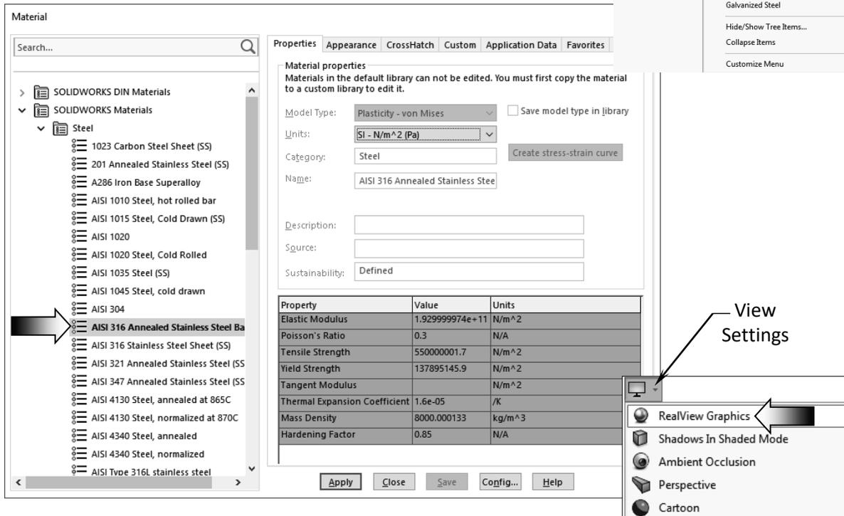
Select the material **AISI Type 316L Stainless Steel Bar** from the list (arrow).
