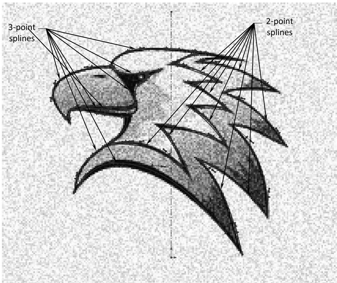
There should be a small gap around the sketch (as noted) so that a single sketch can be extruded into a feature.
