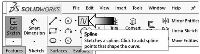
Keep in mind that the simpler the spline, the easier it is to manipulate it. So, we are going to create one spline with two or three spline points each time, and then adjust it to match the outline of the image as close as possible. (Zoom in a little closer.)
