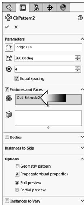
Enable the **Equal Spacing** checkbox.
