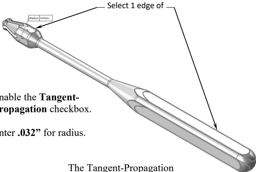
Enable the **Tangent-Propagation** checkbox.
