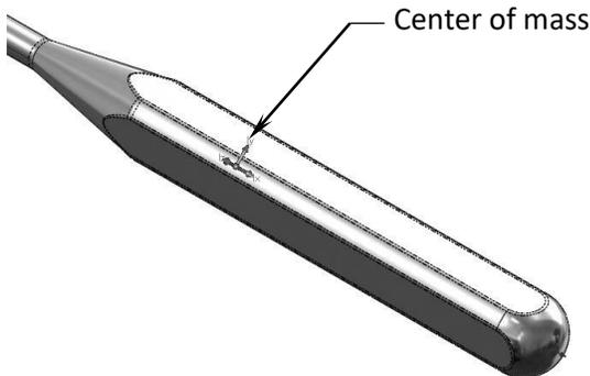
In the graphics area, a single-colored triad indicates the principal axes and center of mass of the model.
