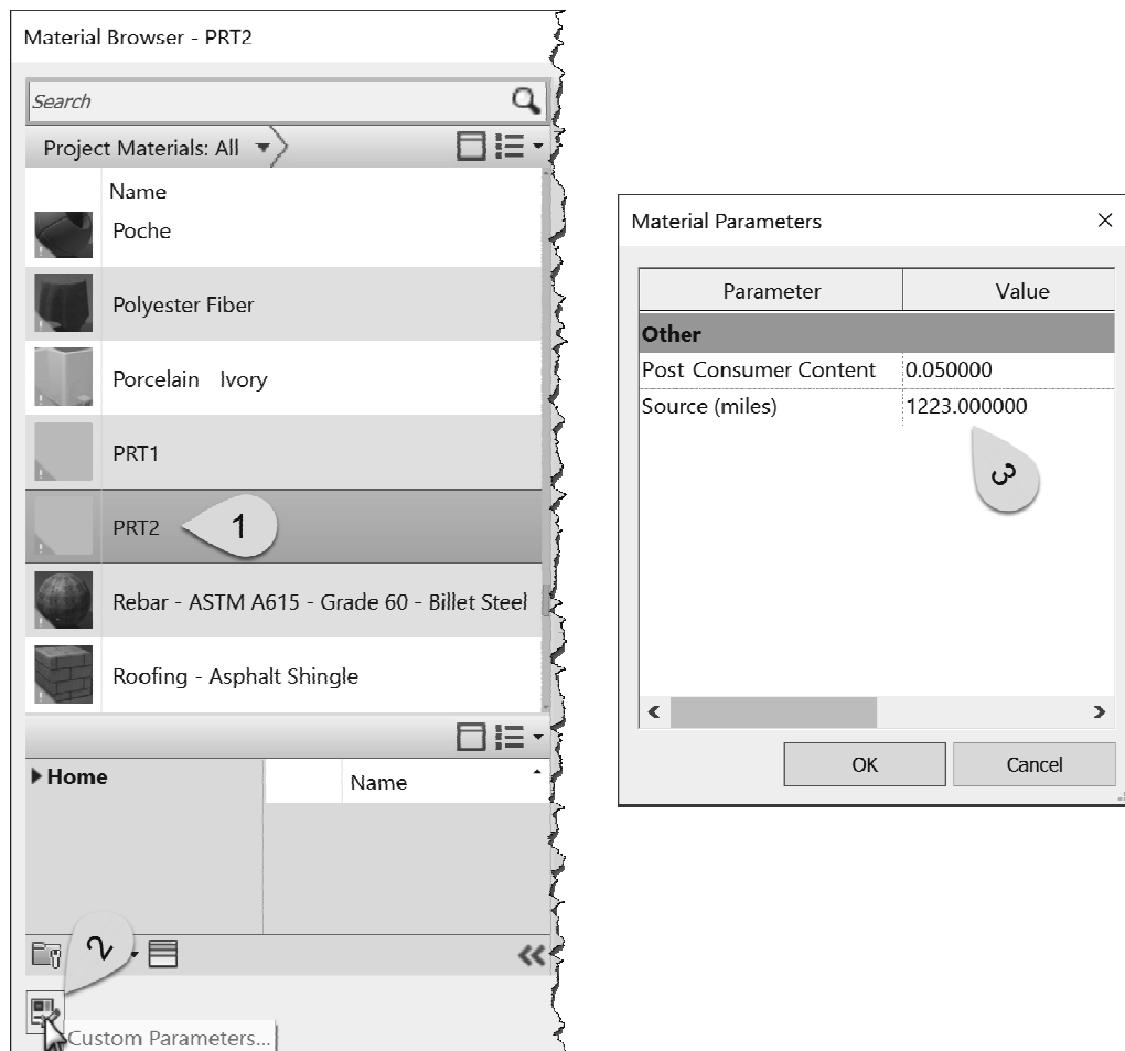
FIGURE 4-5.2 Custom material parameters in the Materials dialog
