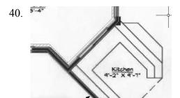
Place interior wall segments in the kitchen area using the interior wall style **Stud-2.5 GWB-0.625 Each Side**.
