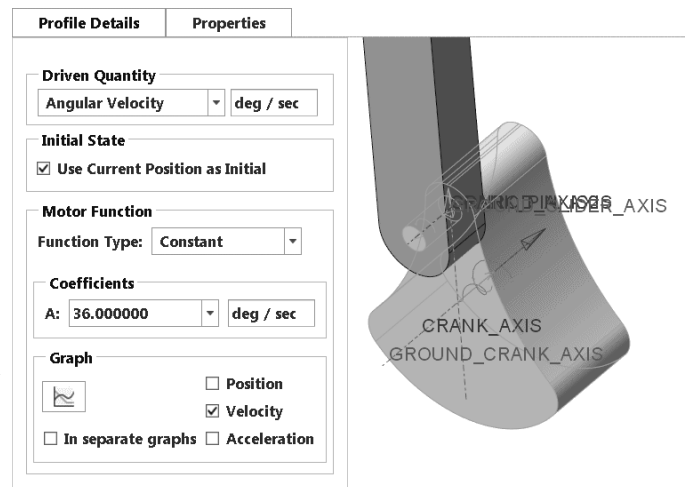
Figure 1 Defining a constant speed servo motor to drive the crank.
