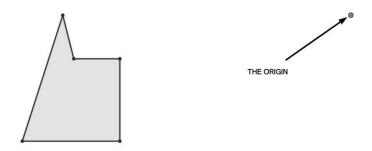
Because the sketch is located in 3-dimensional space, the elements always need to be located in relation to the origin in order to be fully defined. Otherwise, they are just floating in space.
