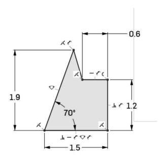
Once the two dimensions are added to indicate where the elements are located relative to the origin, the sketch will display in black – fully defined.
