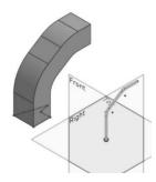
A Loft is also called a blend. A loft is created by placing two or more sketches on offset planes. Each sketch is usually a different shape. The loft blends the sketches together to create a unique 3D feature. Common objects that use lofts are faucets and bottles.
