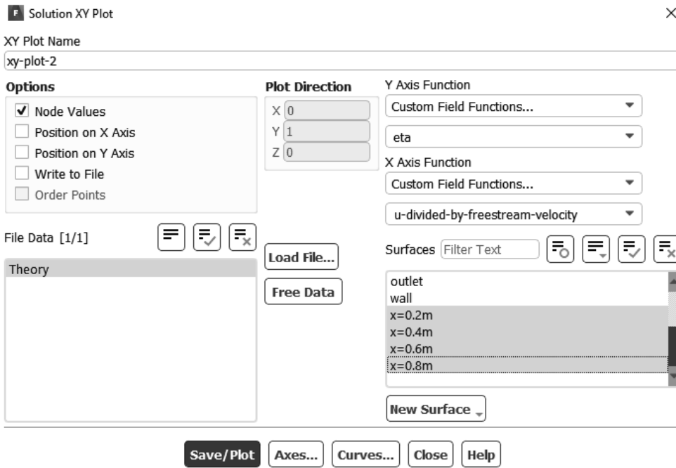
Figure 2.17a) Solution XY Plot for self-similar velocity profiles
