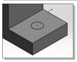
6. Create a circle of arbitrary size on the top face of the solid model as shown. Click once with the left-mouse-button to select the center of the circle, move and click again to set the radius. Press the [Esc] key once to end the Circle command.
