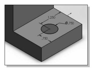
7. On your own, create and modify the dimensions of the sketch as shown in the figure. **NOTE:** Select the center of the circle, then the appropriate edge to apply the linear dimensions. Select any point on the circle to apply the diameter dimension.
