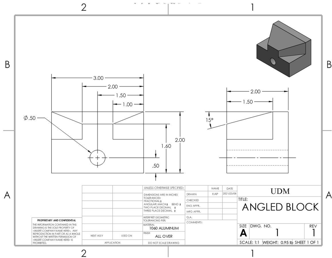
Figure 2.6-1: Angled block detail drawing
