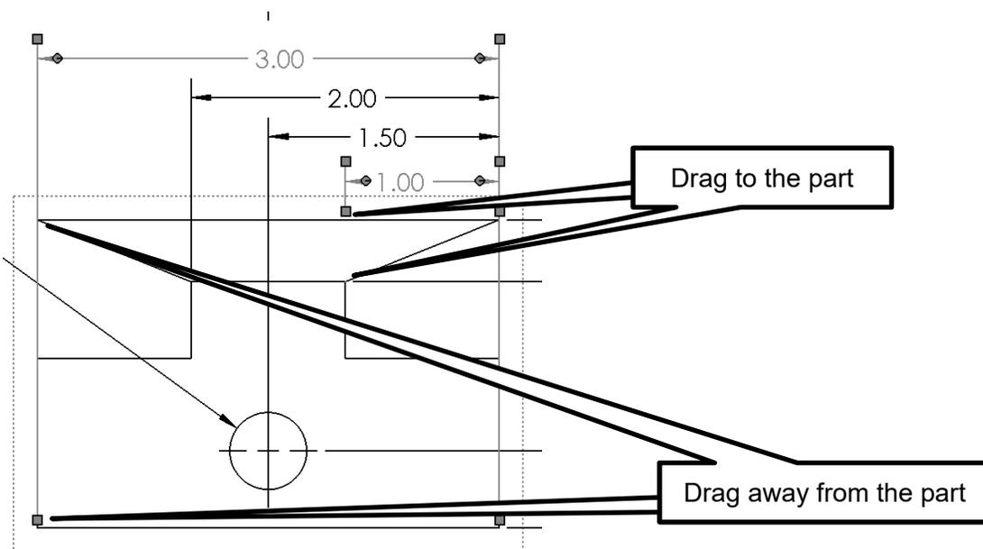
8) Drag the dimensions and the dimension text into the correct locations. Holding the **ALT** key will produce a smooth drag. The final *Front* view should look like the figure.
