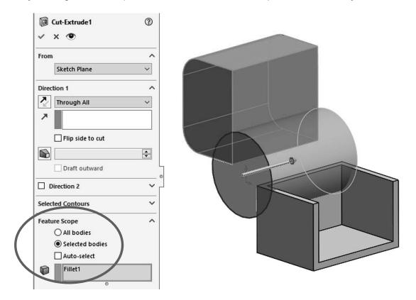
And just as with the features that add material, this technique works the same way with all the features that remove material including revolved cut, sweep cut, loft cut, etc.
