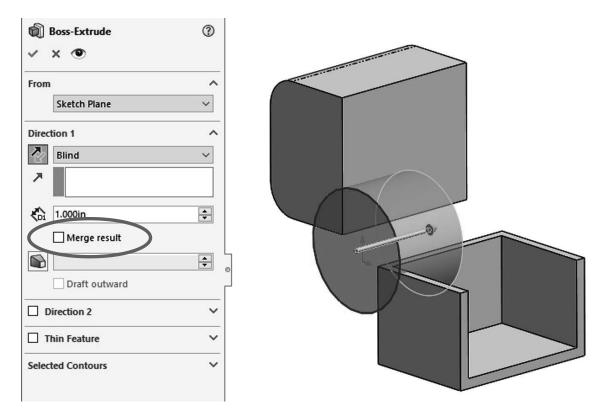
**1.7.** - After adding this extrusion we have three different bodies in our part. See how the different bodies' edges intersect each other. If the "Merge result" option had been checked, we would not see the overlapping edges as they would be merged into a single body.
