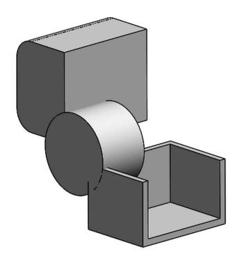
Edit the last extrusion to explore the effect of different "Merge Result" and "Feature Scope" combinations.
