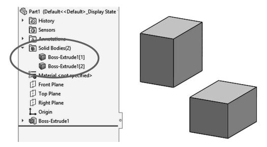
**1.3.** - The next step is to add a new feature. When working in a multi body part we can make 'local' operations to each body, in other words, a feature affecting only one solid body. Local operations are applied features like fillets, shells, chamfers, etc., which can only be applied to a single body at a time; for example, we cannot fillet or shell both bodies at the same time. Select the "**Shell**" command from the Features toolbar and shell the bottom body removing the indicated faces.
