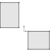
**1.2.** - Select the "**Extruded Boss**" command. Notice that we are not given a warning about having two separate bodies; it just works. Extrude the sketch any size that looks similar to the following image (dimensions are not important at this time) and click **OK** to finish. Making two or more extruded/revolved/swept features would work the same.
