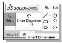
6. Select the **Smart Dimension** command in the *Sketch* toolbar. The Smart Dimension command allows us to quickly create and modify dimensions.
