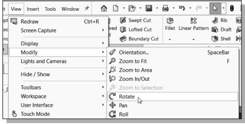
2. Move the cursor inside the graphics area. Press down the left-mouse-button and drag in an arbitrary direction; the Rotate View command allows us to freely rotate the solid model.
