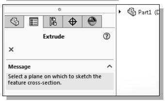
Note the *Extrude Property Manager* is displayed in the left panel. We have activated the extrude feature; *SOLIDWORKS* requires the use of an existing 2D sketch or the creation of a new 2D sketch.
