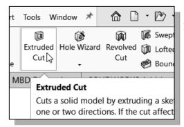
In the *Features* toolbar select the **Extruded** Cut command by clicking once with the left-mouse-button on the icon.
