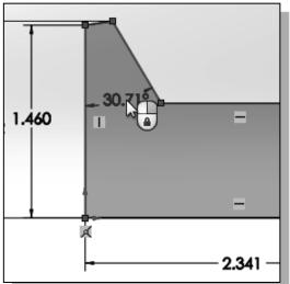
21. Place the angular dimension in the middle of the two selected lines as shown.
