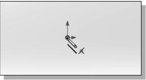
2. Move the cursor on top of the *Origin*, the little coordinate system near the center of the graphics area, and notice the constraint symbol as shown.
