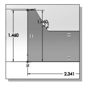
20. Select the longer inclined line on the left as the  $2^{nd}$  geometry to dimension.
