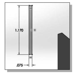
9. Create the two location dimensions, accepting the default values, to describe the position of the sketch relative to the top corner of the solid model as shown.
