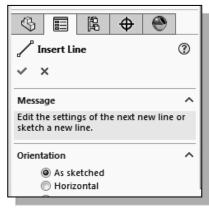
Note the *Insert Line Feature Manager* is displayed in the left panel with different options related to the active command.
