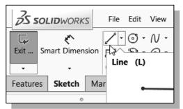
1. Move the graphics cursor to the **Line** icon in the *Sketch* toolbar. A *Help tip* box appears next to the cursor and a brief description of the command is displayed at the bottom of the drawing screen: "*Sketches a line*." Select the icon by clicking once with the **left-mouse-button**.
