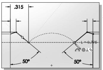
3. Select the endpoint of the longer inclined line on the right as shown.
