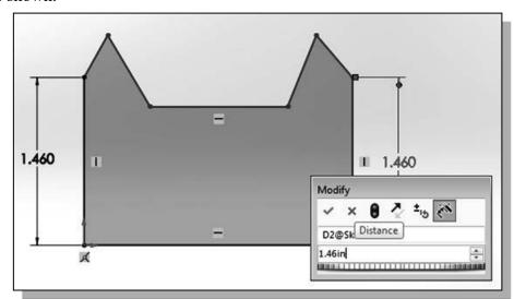
❖ The Smart Dimension command will create a length dimension if a single line is selected.
