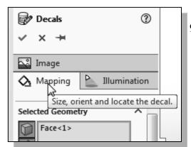
9. Switch to the **Mapping** options by clicking on the associated tab as shown.
