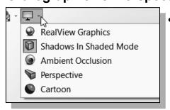
• Besides the basic display modes, we can also choose an orthographic view or perspective view of the display. Clicking on the View Settings icon on the *Heads-up View* toolbar will reveal the Perspective icon. Clicking on the Perspective icon toggles the perspective view *ON* and *OFF*.
