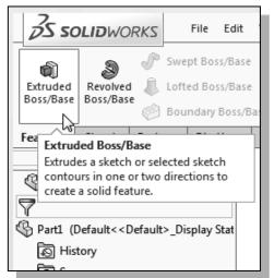
1. In the *Features* toolbar select the **Extruded Boss/Base** command by clicking once with the left-mouse-button on the icon.
