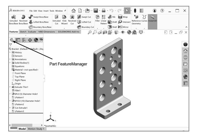
The FeatureManager design tree is located on the left side of the SOLIDWORKS Graphics window. The FeatureManager provides a summarized view of the active part, assembly, or drawing document. The tree displays the details on how the part, assembly or drawing document was created.
