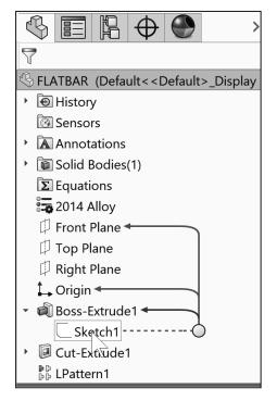
Use Dynamic reference visualization for a part, assembly and mates.
