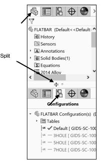
The ConfigurationManager tab is located to the right of the PropertyManager 🔳 tab. Use the ConfigurationManager to create, select and view multiple configurations of parts and assemblies.
