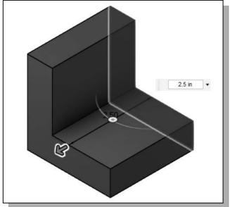
4. In the *Extrude* edit box, enter **2.5** as the extrusion distance.
