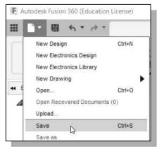
1. Select **Save** in the *Quick Access* toolbar, or you can also use the "**Ctrl-S**" combination (hold down the "**Ctrl**" key and hit the "S" key once) to save the part.
