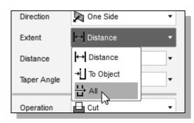
15. Set the *Extent* option to **Through All** as shown. The *All* option instructs the software to calculate the extrusion distance and assures the created feature will always cut through the full length of the model.
