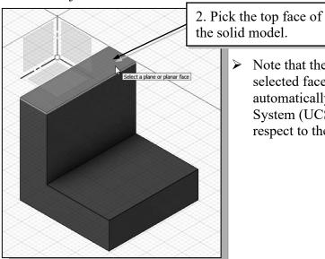
Note that the sketch plane is aligned to the selected face. Autodesk Fusion 360 automatically establishes a User-Coordinate-System (UCS) and records its location with respect to the part on which it was created.
