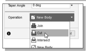
12. Select the **CUT** option in the *feature option* list to set the extrusion operation to *Cut*.
