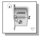
9. Move the cursor over one of the corners of the ViewCube and drag with the left-mouse-button to activate the **Free Rotation** option.
