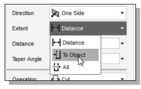
11. Set the *Extents* option to **To Object** as shown. The *To Object* option instructs the software to calculate the extrusion distance and assures the created feature will always cut through the proper length of the model.
