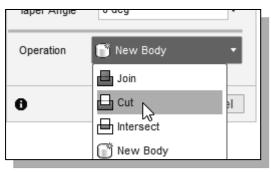
10. Select the **CUT** option in the *feature option* list to set the extrusion operation to *Cut*.
